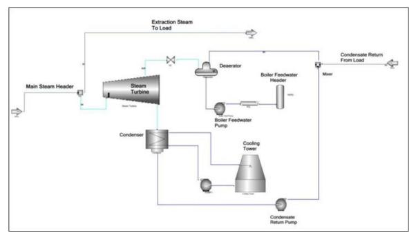
Figure 4. CHP main steam extraction
