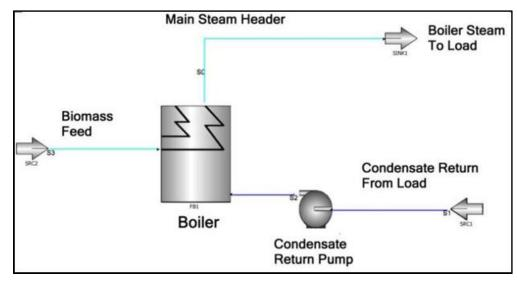
Figure 2. Thermal-only biomass energy system
