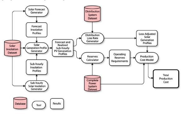
Figure 5. Schematic flow diagram of a PCM run used to calculate energy value of DGPV, including impact of added reserves
