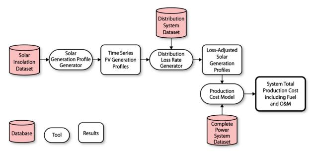
Figure 2. Schematic flow diagram of a PCM run used to calculate energy value of DGPV
