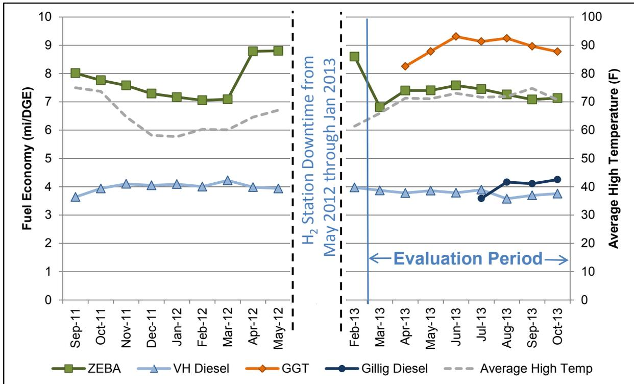
Figure 17. Average fuel economy for the fuel cell and diesel buses (evaluation period)
