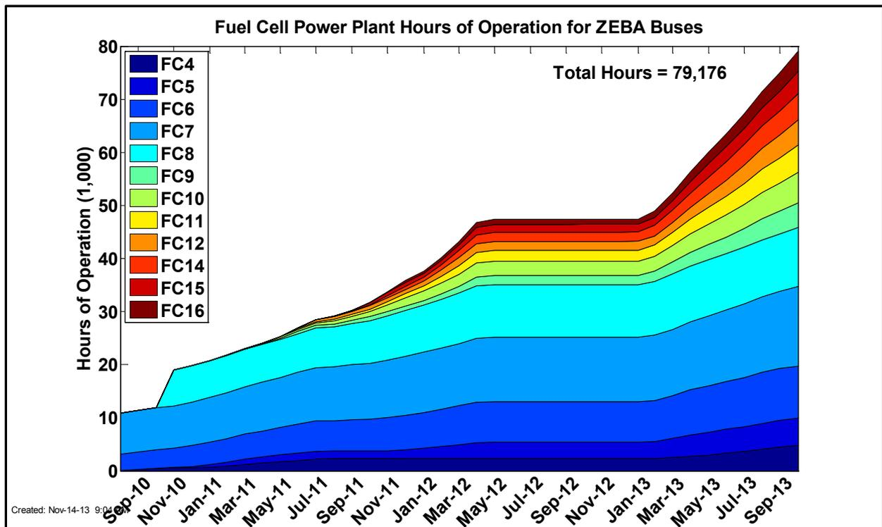
Figure 14. Cumulative FCPP hours on the ZEBAs buses
