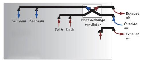
The compartmentalization strategy of using a separate HRV in each apartment unit results in a much smaller and more compact distribution system. The HRV will be located in a mechanical closet in each apartment and the common areas. A small duct system will provide ventilation to the bedrooms and will draw stale air from the bathrooms.
