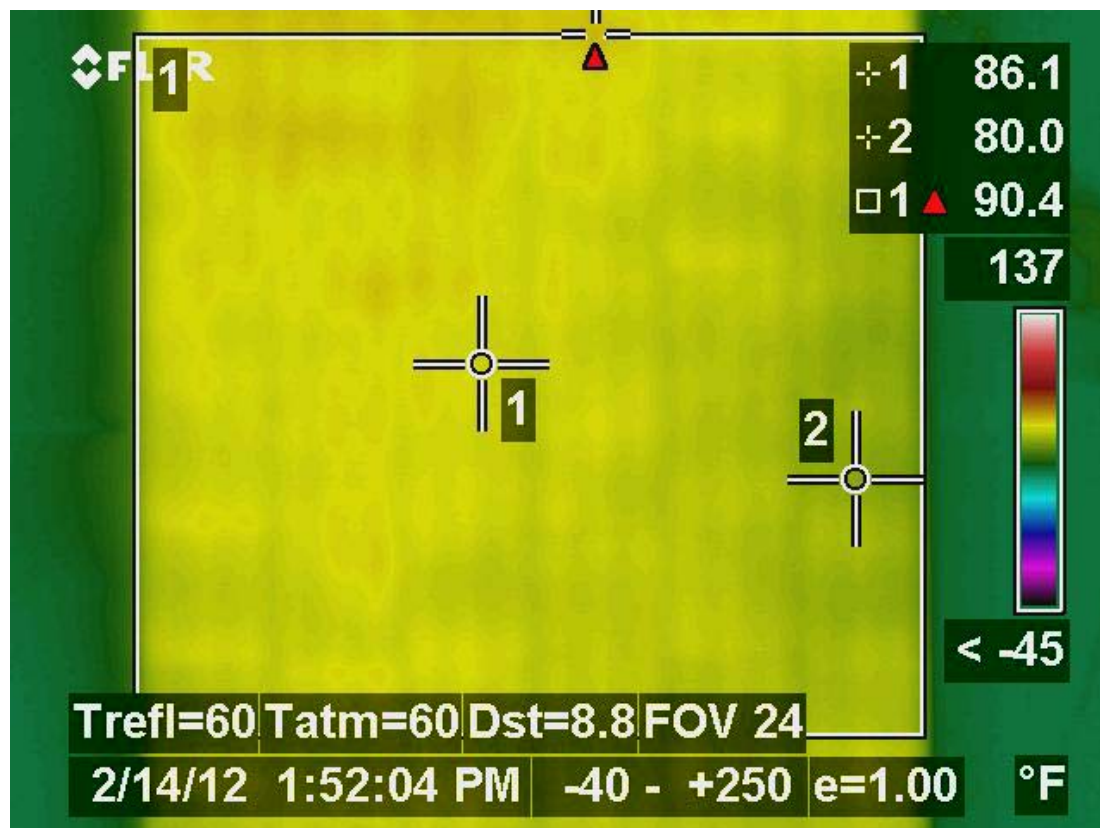
Figure 8. IR Image of 235 Watt Solar Module
