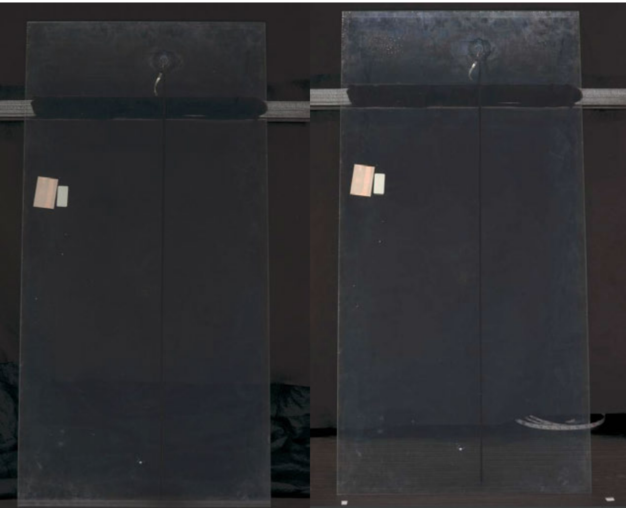
TPU after 100°C No Creep Pass Wet Hi-Pot
