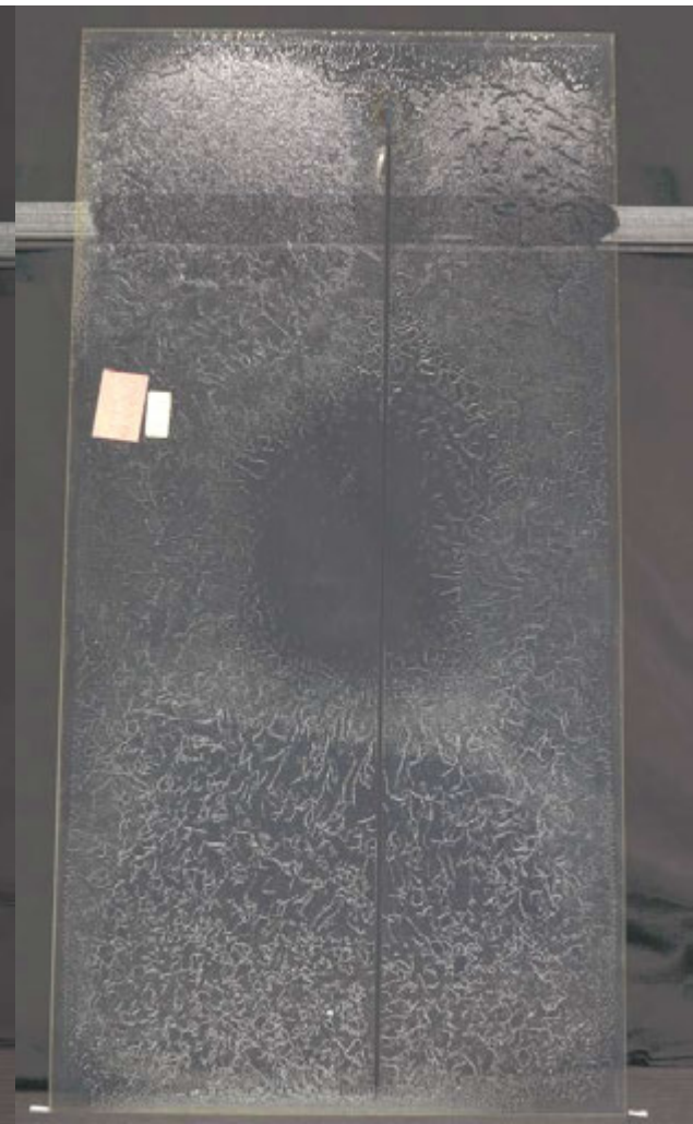
TPU after 120°C 0.482 mm Creep Pass Wet Hi-Pot
