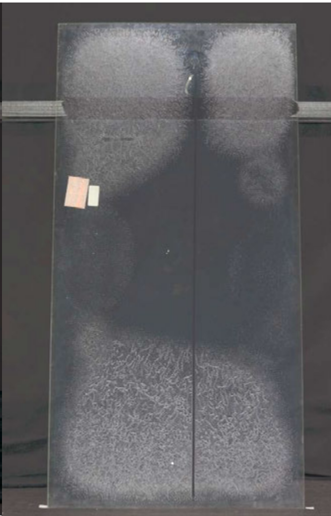
TPU after 110°C 0.023 mm Creep Pass Wet Hi-Pot
