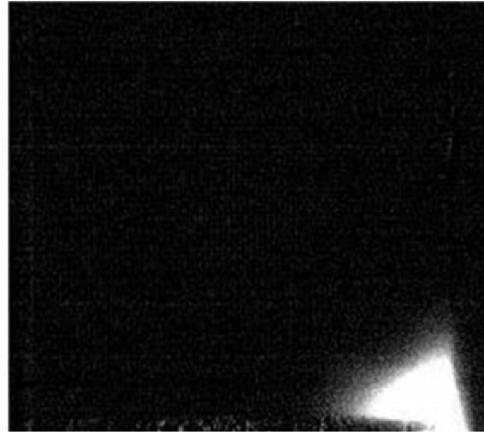
Steady-state IR image showing shunt caused by sun exposure
