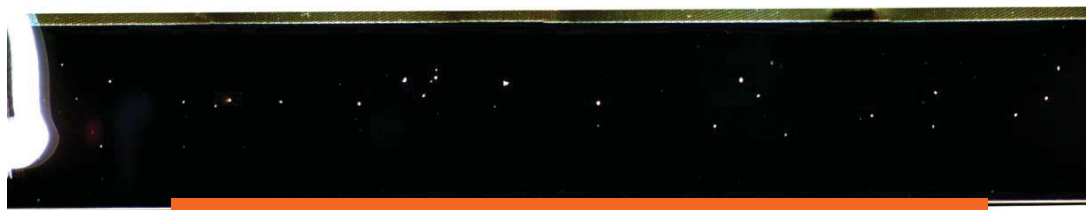
Film damage at burned conduction points
