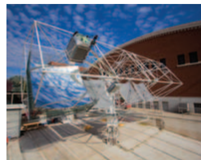
Figure 4: 20kW Solar Tracker Unit
