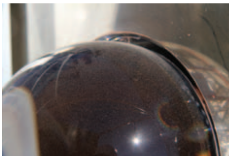
Figure 3: Dust Accumulation on Ball Lens
