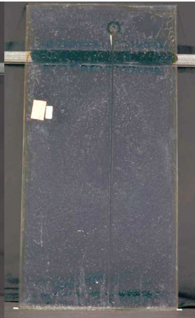
TPU after 130°C >1 cm Creep Fail Wet Hi-Pot
