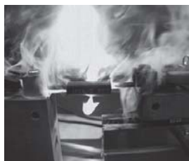
Sleeve of PV cable type "USE2" during burn-through test at 7 A
