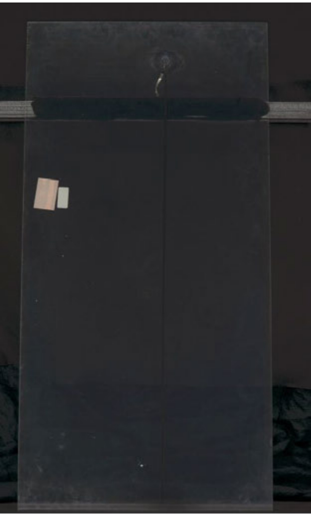
TPU after 100°C No Creep Pass Wet Hi-Pot
