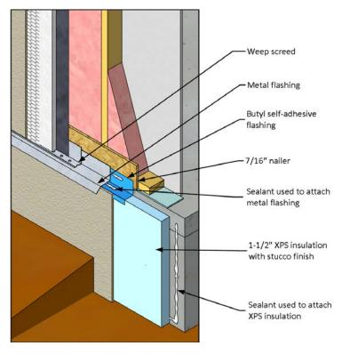
Construction detail showing key parts of the slab edge insulation flashing.
