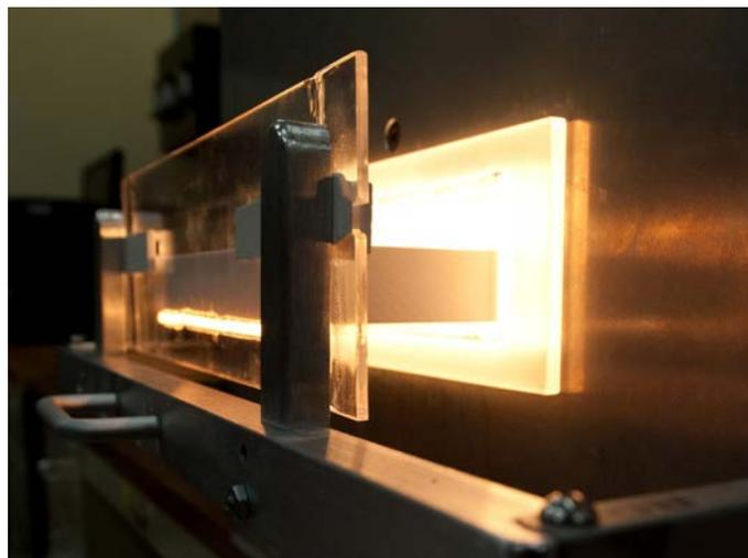
The cavity inside the OCF glows white hot during a simulated firing of a solar cell.
