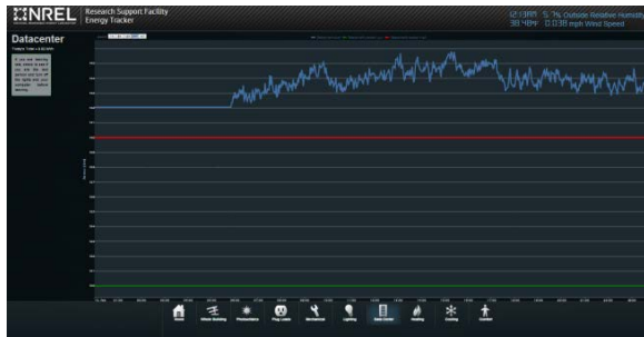
Figure 4: BA Dashboard for the RSF (data centre power consumption (kW), February 13, 2013, energy use not within predicted range)
