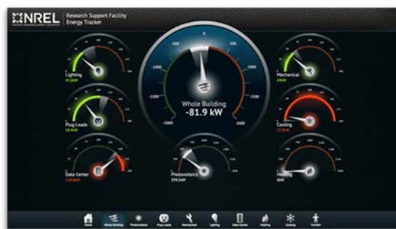
Figure 3: BA Dashboard for the RSF (whole building, May 15, 2013, partly cloudy day)
