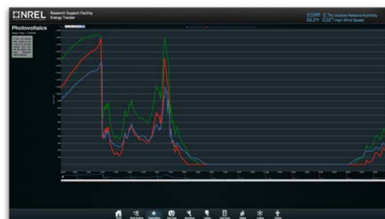
Figure 6: PV Production Predicted Range Visualisation (May 15, 2013, partly cloudy day)
