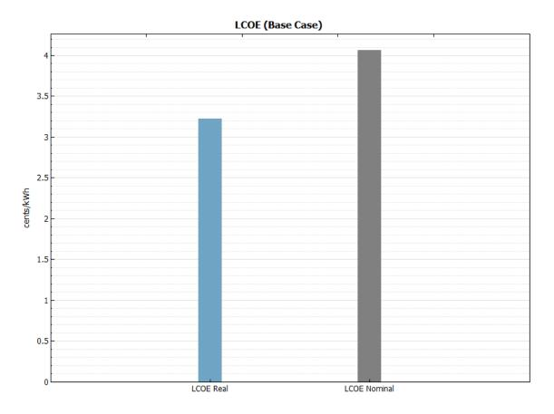
Figure B-7. LCOE for 2-MW net-metering fixed-axis system
