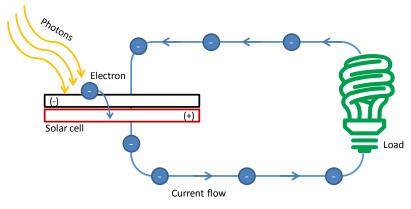
Figure 1. Generation of electricity from a PV cell Source: EPA
