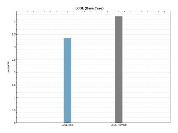
Figure B-11. LCOE for a 2-MW net-metering system single-axis tracking PV system
