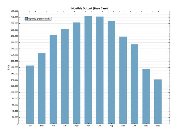
Figure B-3. Modeled output for 2-MW net-metering single-axis tracking PV system
