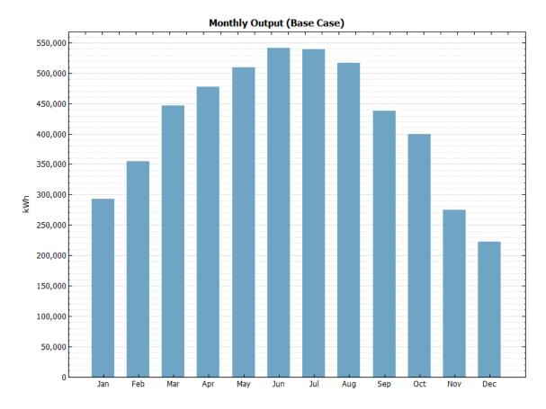
Figure B-2. Modeled output for full coverage single-axis tracking PV system
