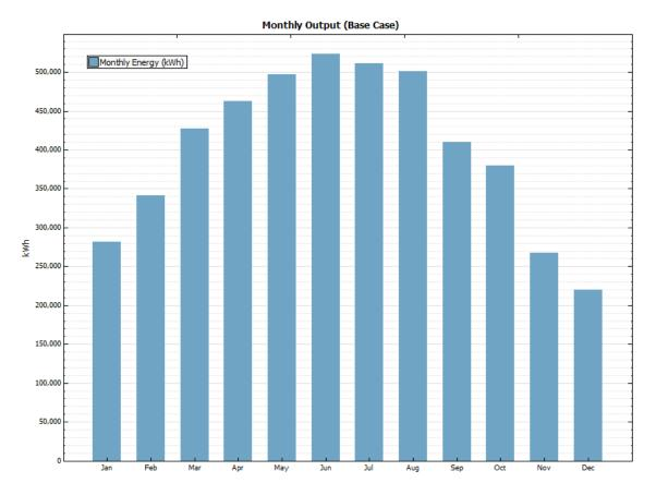
Figure B-1. Modeled output for full coverage fixed-axis ground system
