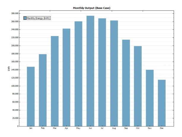
Figure B-4. Modeled output for 2-MW net-metering fixed-axis PV system
