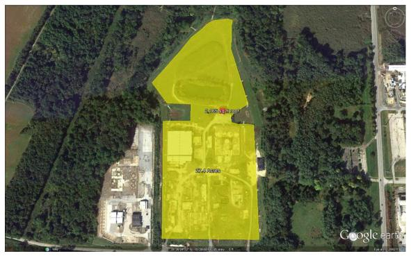
Figure 6. Aerial view of the feasible areas for PV at the Standard Chlorine of Delaware site (ground-mounted PV in yellow and treatment system building with roof-mounted PV in red)
