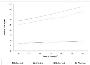
Fig. 6. Reverse characteristics of diodes 2-2(Q2) and diode 3-2(Z2) before and after thermal cycle plus reverse bias testing
