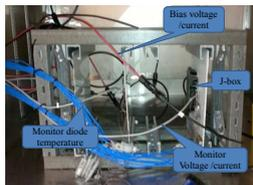
Fig. 2. Assembled testing samples in the chamber
