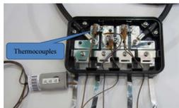
Fig. 1. Junction box sample for testing
