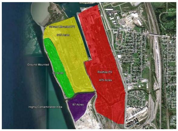
Figure 6. Aerial view of the feasible areas for PV at the Former Bethlehem Steel Plant (ground-mounted micro-inverter PV in green; ground-mounted PV in yellow; light industrial rooftop PV in red; highly contaminated area in purple)
