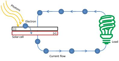
Figure 1. Generation of electricity from a PV cell Source: EPA
