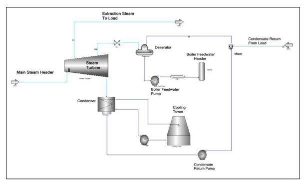
Figure 7. CHP extraction turbine
