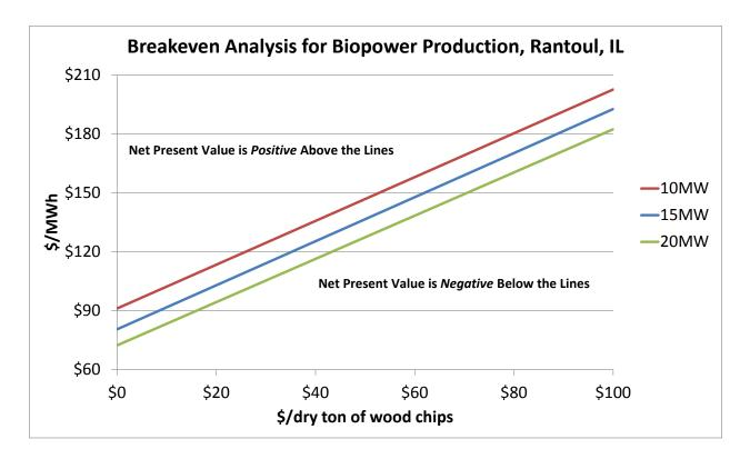
Figure ES-1. Breakeven analysis for biopower production at 10-MW, 15-MW, and 20-MW scales
