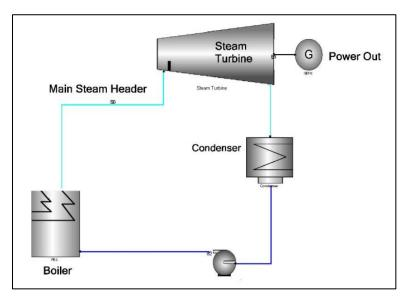
Figure 5. Power generation only biomass energy system (cooling tower not shown) Source: Gregg Tomberlin, NREL
