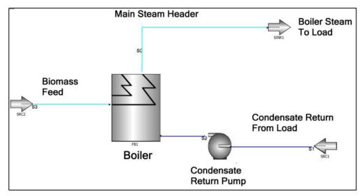
Figure 4. Thermal only biomass energy system
