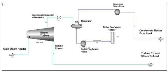
Figure 8. CHP backpressure turbine
