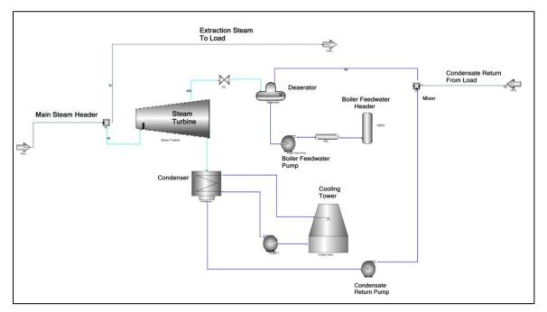
Figure 6. CHP main steam extraction
