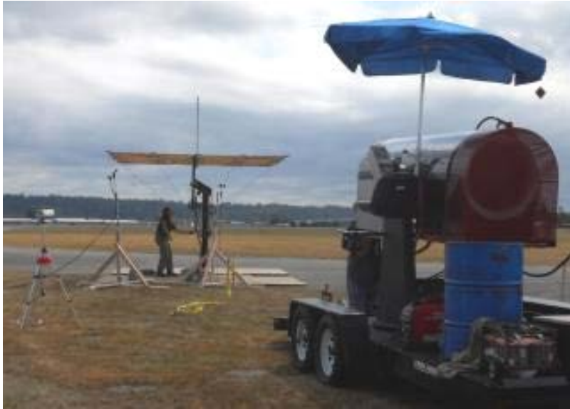
Figure 11 Testing Heliostat with Jet Engine
