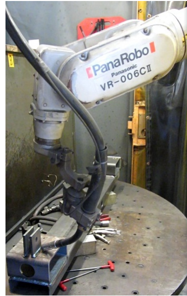
Figure 5 Robotic Welder on Elevation Assembly
