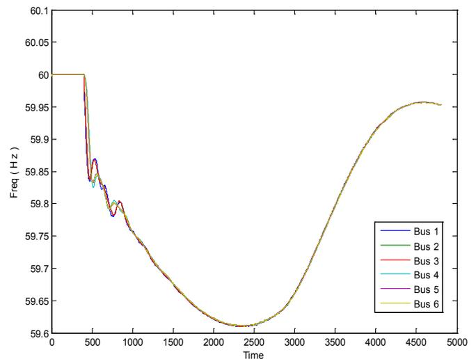
**Figure 7** Frequency responses at six wind generator buses
