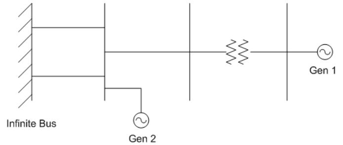
Figure 2 Two-machine infinite bus system diagram
