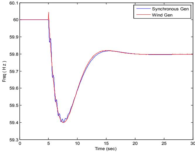
**Figure 4** Frequency response comparison between a synchronous generator and a wind generator
