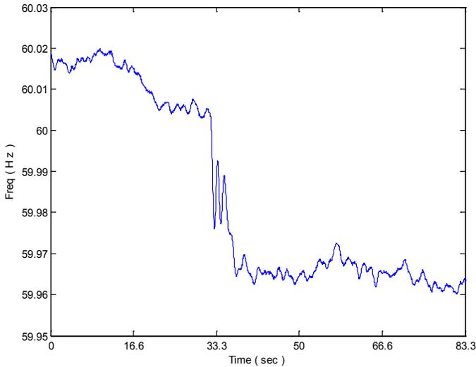
Figure 11 Frequency response at a wind generator bus
