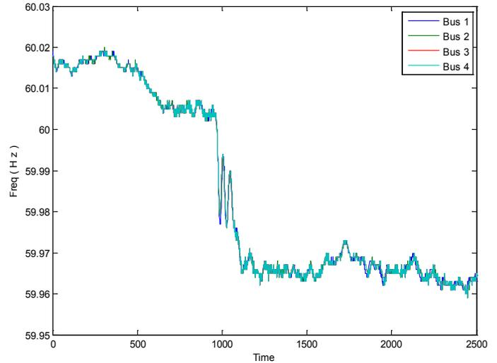
**Figure 9 Frequency responses at four buses from PMUs**
