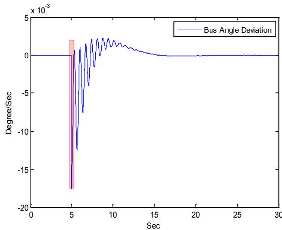
Figure 1 Time window for inertial estimation
