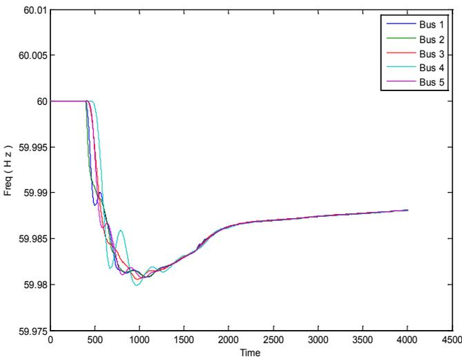
**Figure 5** Frequency responses at five synchronous generator buses
