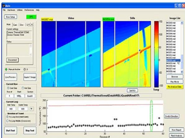
*Thermal Scout's user-friendly data acquisition interface allows users to read data in real time or save it for later analysis. The left screen shows a video image with the mirrors in blue and the tube in lighter blue. The right side shows a still shot with the tube in orange. In the space below, a series of dots shows which tubes have elevated temperatures.*
