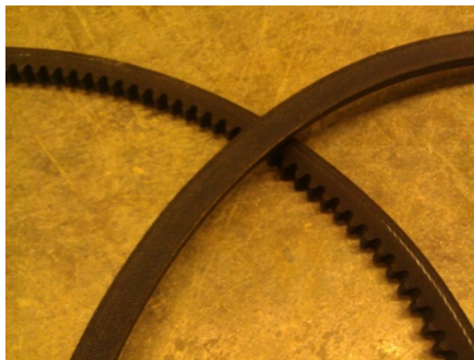
Figure 24. Cogged V-belt (left) and standard V-belt (right) Photo by Caleb Rockenbaugh, NREL
