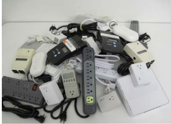
Figure 10. Example of various plug load control devices
