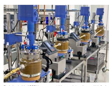
Berkeley Lab's ABPDU can convert biomass into advanced biofuels for engine testing. Photo from Roy Kaltschmidt, photographer, Lawrence Berkeley National Laboratory
