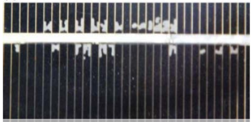
Semiconductor/Encapsulant delamination near busbar
