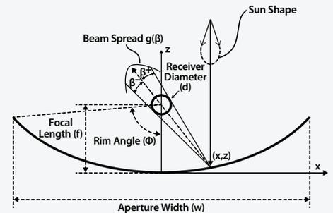
*Simplified representation of a parabolic trough collector. Note that the receiver size and the sun shape are exaggerated for demonstration purposes. Illustration by Guangdong Zhu, NREL*
