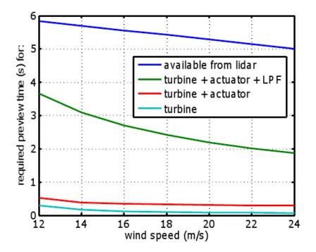
Figure 18. Cumulative required preview times for the turbine, actuator, and lowpass filter (LPF). Available preview time from the LIDAR is also shown.
