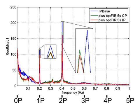
Figure 13. Blade root bending moment as a function of frequency. If x is the root bending moment in-plane and y is out-of-plane, then the plot is  $\sqrt{x^2 + y^2}$ . Average FFT magnitude over AR1\_s12 through AR1\_s27.
