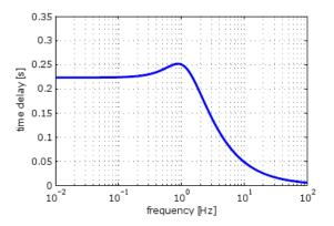
Figure 20. Time delay of second-order actuator model (natural frequency 1 Hz, damping ratio 0.7) time delay = -(phase from Figure 19)/(360 degrees)/(frequency)
