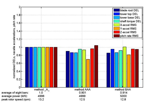
Figure 9. Turbine loads using individual pitch baseline control (A) alone, [5] with added individual pitch feedforward controller A, and with added individual pitch feedforward controller B. The rated rotor speed is 12.1 rpm, and the rated power is 5,000.0 kW. X-accel, Y-accel, and Z-accel are respectively fore-aft, side-to-side, and up-down nacelle accelerations. The wind field used is the IEC Kaimal NTM spectral model with a Class A turbulence level, at 14 m/s average wind speed.
