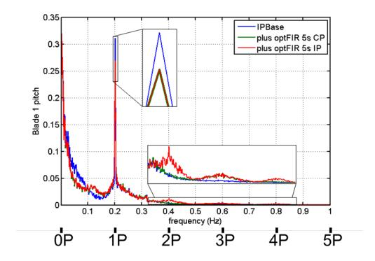
Figure 15. Blade pitch angle as a function of frequency. Average FFT magnitude over AR1\_s12 through AR1\_s27.
