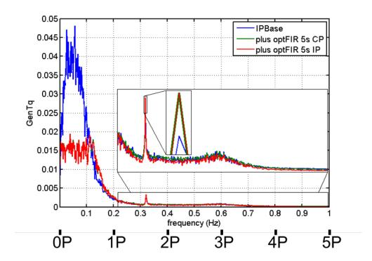
Figure 16. Generator torque as a function of frequency. Average FFT magnitude over AR1\_s12 through AR1\_s27.
