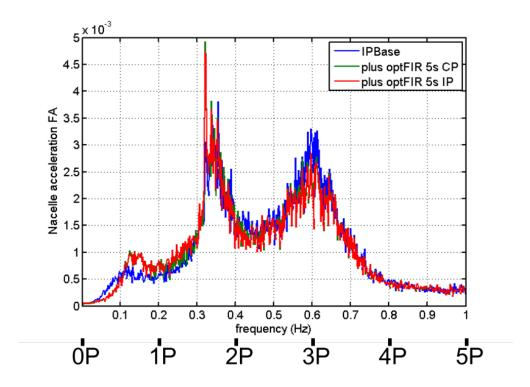
Figure 14. Fore-aft nacelle acceleration as a function of frequency. Average FFT magnitude over AR1\_s12 through AR1\_s27.
