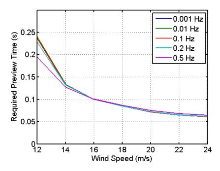
Figure 23. Estimated required preview time due to the turbine itself. Five degrees of freedom turned on in linearization: first flapwise blade mode (×3 blades), generator, and drivetrain rotational-flexibility.
