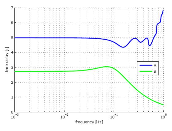
Figure 11. Time delay of feedforward controllers A and B time delay = -(phase from Figure 10)/(360 degrees)/(frequency)
