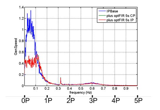
Figure 17. Generator speed as a function of frequency. Average FFT magnitude over AR1\_s12 through AR1\_s27. (This subset of the wind fields was chosen arbitrarily due to computer memory limitations).
