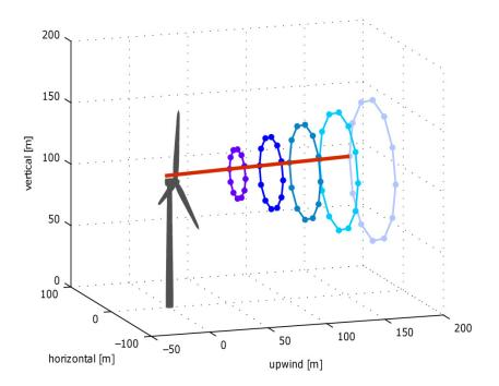
Figure 6. LIDAR configuration B pulsed LIDAR scanning pattern
