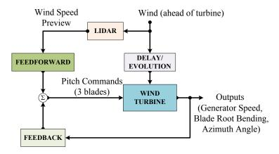
Figure 1. Feedforward control added to feedback control
