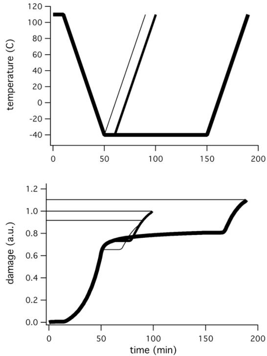
FIGURE 1. Temperature profiles and simulated accumulated damage for varying cold dwell times.
