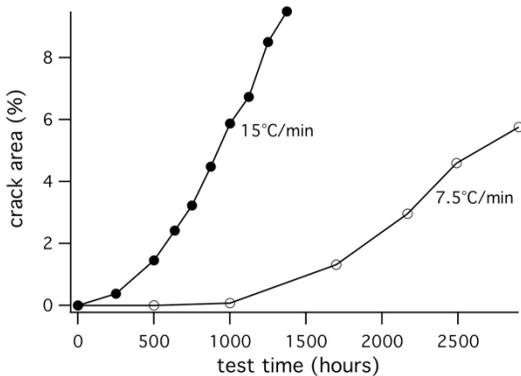
FIGURE 8. Crack growth vs. test time.
