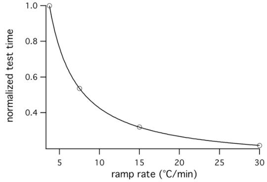
**FIGURE 4.** Normalized test time for increasing temperature ramp rates.
