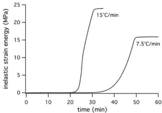
**FIGURE 6.** FEM simulated accumulation of inelastic strain energy (damage) for the two experimental thermal cycles.
