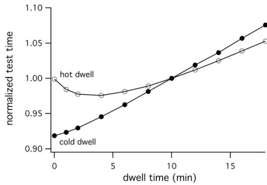
**FIGURE 5.** Normalized test time for increasing hot and cold dwell times.
