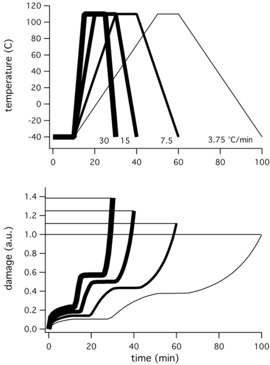
**FIGURE 3.** Temperature profiles and simulated accumulated damage for varying ramp rates.
