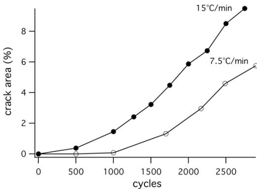
FIGURE 7. Crack growth vs. number of cycles.
