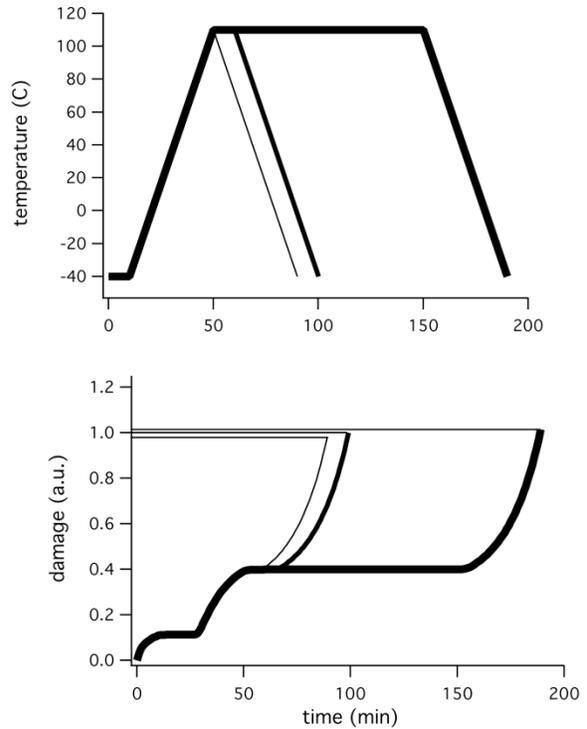
FIGURE 2. Temperature profiles and simulated accumulated damage for varying hot dwell times.
