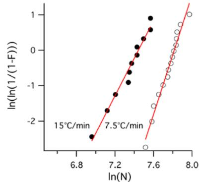
FIGURE 9. Weibull plot of die attach failure.
