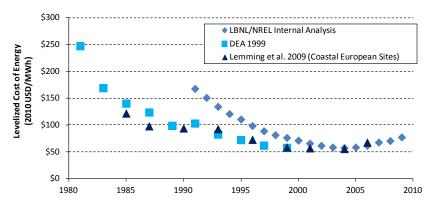
Fig. 3: Estimated LCOE for wind energy between 1980 and 2009 for the United States and Europe (excluding incentives); Sources: LBNL/NREL (internal analysis), [3-4].
