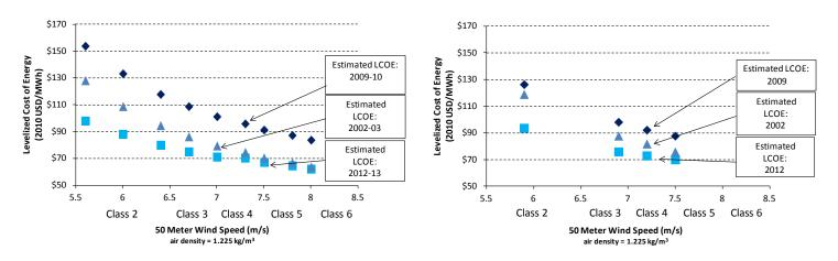
Fig. 4: LCOE for wind energy over time in the United States (left) and Denmark (right) [10-11].
