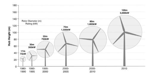
Fig. 2: Representative turbine architectures from 1980 to 2010; Source: NREL.
