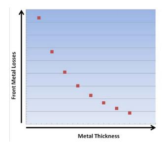
To the left is a graph showing the dependence of front contact losses on the metal thickness. The detailed numbers depend on exact device and cell designs, but in general, thicker metal is favorable. Electroplating through patterned resist is a process that can deliver narrow line width and thick metal. Prior to plating, Alta utilized a lift-off metallization process, which addresses the narrow line width requirement, but is limited to very small thicknesses.
