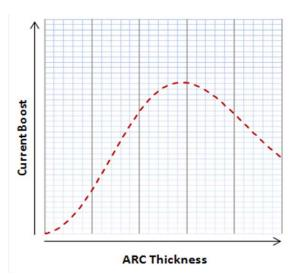
performance. Altogether, the thickness, refractive index, and number of layers impact the final performance with the main performance indicator being the short-circuit current (Isc.) Measurements of Isc before and after ARC deposition are representative of the amount of light reaching the solar cell junction. The graph on the left shows how current boost (defined as Isc post-ARC minus Isc pre-ARC) depends on the ARC thickness.
