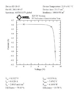
Deliverable D-13: Sub-modules with area  $> 0.02 \text{ m}^2$  and efficiency > 16%
