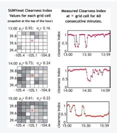
Variability in the clearness index—a ratio of the actual-to-expected insolation—is visualized as a snapshot in time across a region (left). NREL relates the spatial variability to time series irradiance measurements (right) at a single site (red star).
