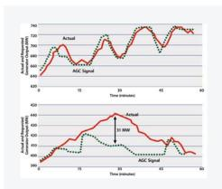
Two coal-fired generators in the Midwest illustrate a difference in ability to follow an automatic generation control signal. The upper generator is providing regulation, while the lower generator is imposing a regulation burden on the power system.
