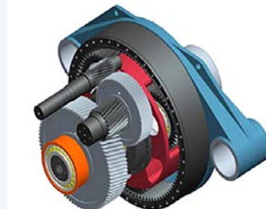
The GRC gearbox has a low-speed planetary stage and two parallel stages. Illustration by Ed Hahlbeck, Powertrain Engineering for NREL
