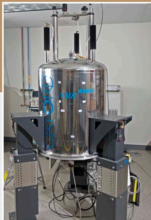
This 400 MHz spectrometer is available to all NREL scientists. Photo by Dennis Schroeder, NREL 19989
