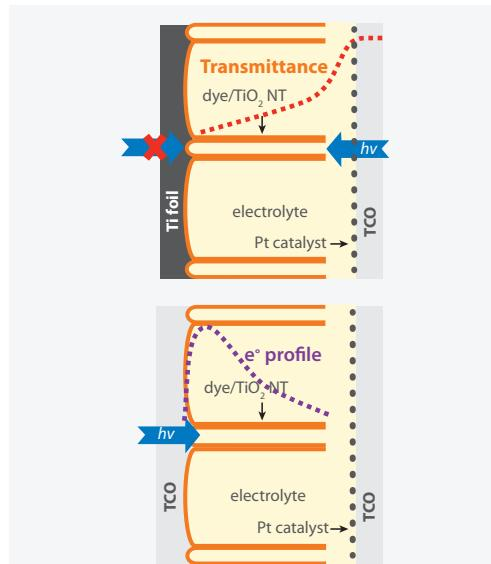
*Illuminating the NT-based DSSC from the photoelectrode side substantially increased the conversion efficiency compared with illuminating it from the counter-electrode side. Back-side illumination (top image) shows light loss by the counter electrode and electrolyte. Front-side illumination (bottom image) shows higher electron density near the current collector.*
