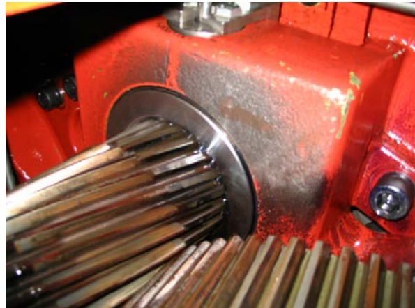
Figure 13. Gearbox 1 high speed stage (taken in field after second oil loss event). PIX #19600.
