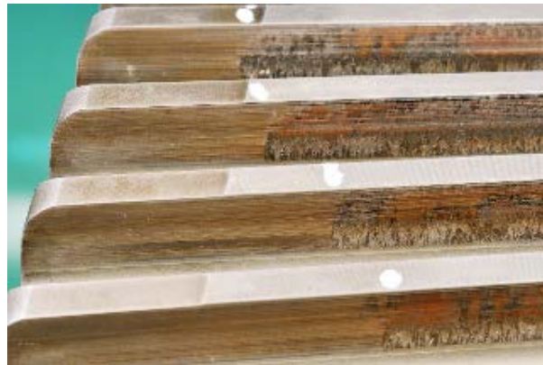
Figure 14. Gearbox 1 high speed stage gear damage (during Gearbox 1 disassembly). PIX #19599.
