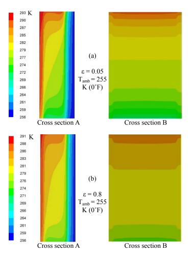
**Figure 2** Effect of surface emissivity,  $\varepsilon$ , on the temperature distribution in the wall when the outdoor ambient temperature is 255 K (0°F).
