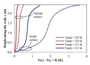
**Figure 4** Temperature profile along the vertical symmetry line of the internal and external surfaces of the wall. The graph shows changes in temperature relative to the bottom of the wall with an emissivity,  $\varepsilon$ , of 0.8.
