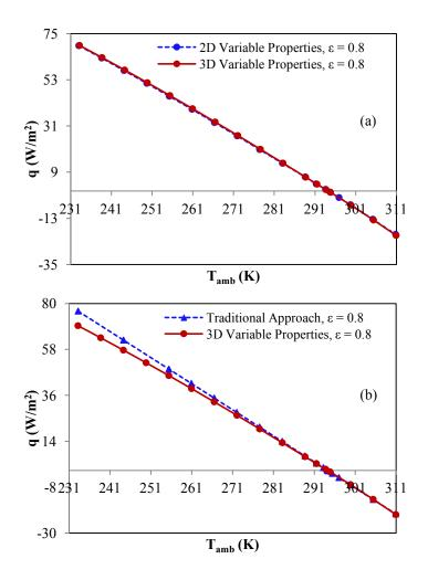
**Figure 9** Total heat flux through the wall assembly as a function of  $T_{amb}$  when the surface emissivity is 0.8. (a) comparison of 3D with 2D and (b) comparison of 3D with the traditional approach, assuming constant resistance evaluated at 297 K (75°F) mean temperature.
