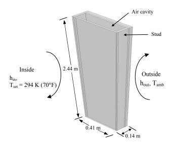
Figure 1 Schematic of the wall structure, which consists of a 0.41-m (16-in.) long  $\times 0.14$ -m (5.5-in.) wide  $\times 2.44$ -m (8-ft) high section of a standard  $2 \times 4$  residential stud wall.
