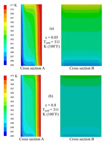
**Figure 3** Effect of surface emissivity,  $\varepsilon$ , on the temperature distribution in the wall when the outdoor ambient temperature is 311 K (100°F).
