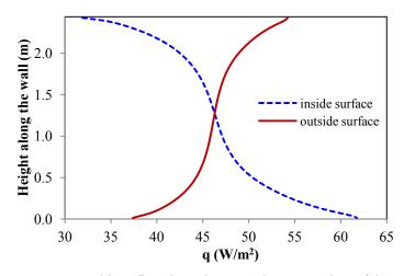
**Figure 5** Local heat flux along the vertical symmetry line of the internal and external surfaces of the wall with an emissivity,  $\varepsilon$ , of 0.8 when the ambient temperature is 255 K (0°F).
