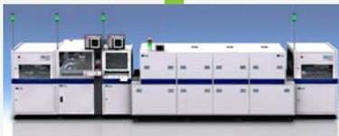
The Silicon Ink printing step uses a readily available commercial screen printer that meshes neatly and without disruption into an existing solar cell production line.
