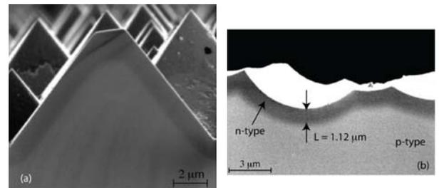
These NREL-produced scanning electron micrographs show the dopant contrast of (a) pyramid and (b) iso-textured wafers; high uniform doping from the Silicon Ink printing process was verified.
