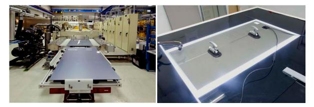
Figure 5. CdTe process equipment exit and a completed module in J-V testing.
