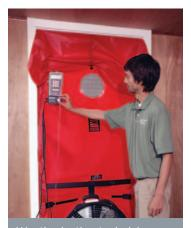
Weatherization technicians use the blower door test to diagnose air leakage problems in a home. Photo from New River Center for Energy Research and Training
