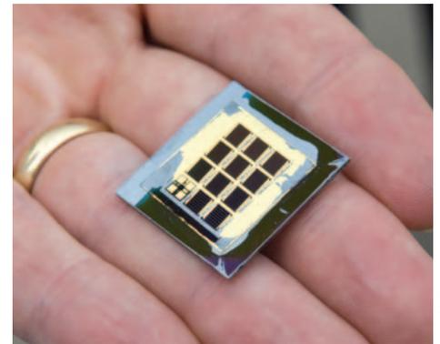
*The IMM solar cell boasts a light weight and high flexibility, as well as an ultra-high efficiency, making it optimal for space and concentrated terrestrial applications. Credit: Patrick Corkery, NREL*
