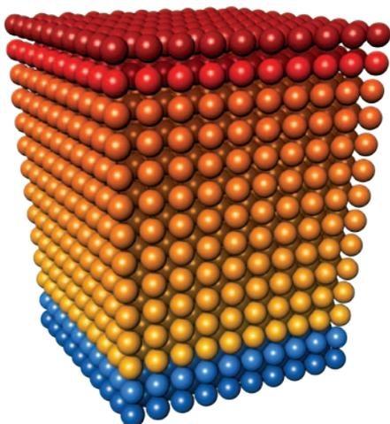
*To build a solar cell from two materials with different lattice spacings, such as gallium arsenide (shown in blue) and gallium indium phosphide (shown in red), the IMM solar cell incorporates a metamorphic layer that gradually changes in composition, creating a transition between the mismatched materials.*
