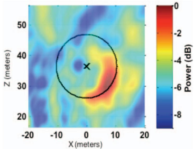
This radar-like picture of the sounds a 100kW wind turbine blade creates shows the loudest region at the apex of the blade rotation in a half-moon shape.
