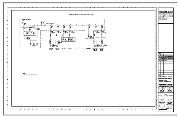
Figure E-1. The 1200-amp main distribution and metering panel "MDP" at the existing treatment plant—with spaces for possible PV tie-in
