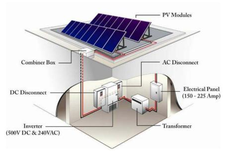
Figure 1. Major components of grid-connected photovoltaic (PV) system
