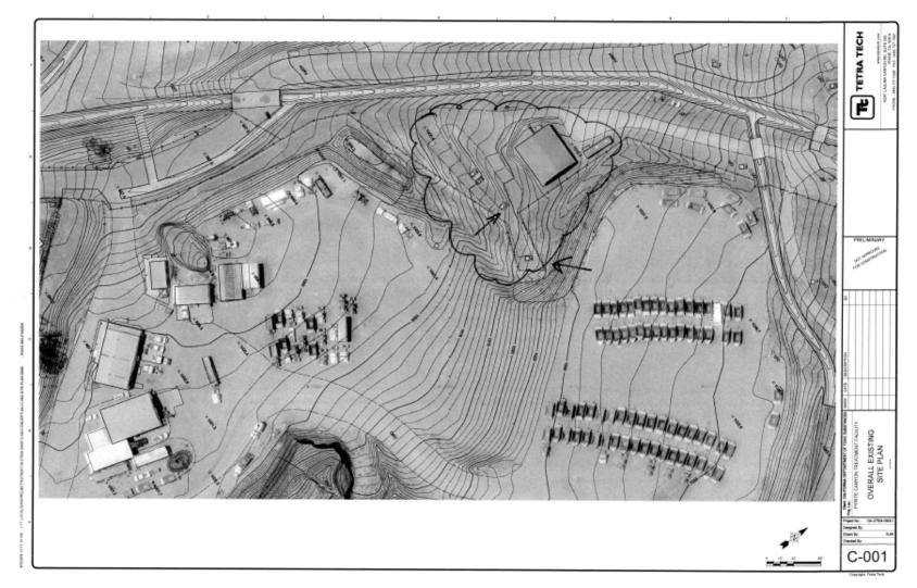
Figure 4. Existing site plan showing topographic contours and proposed PV location in center and east portion of truck parking area Credit: California Department of Toxic Substances Control and Tetra Tech Inc.
