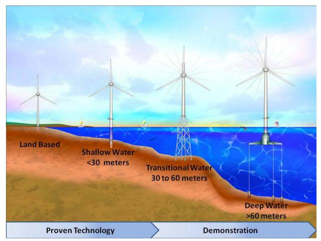
Figure 1-3. Status of offshore wind energy technology
