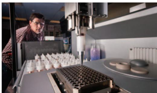
*NREL's custom-designed reactor system, a high-throughput pretreatment and enzyme digestion system, allows researchers to more rapidly screen large numbers of samples to identify the most promising biomass feedstocks. PIX 17132*
