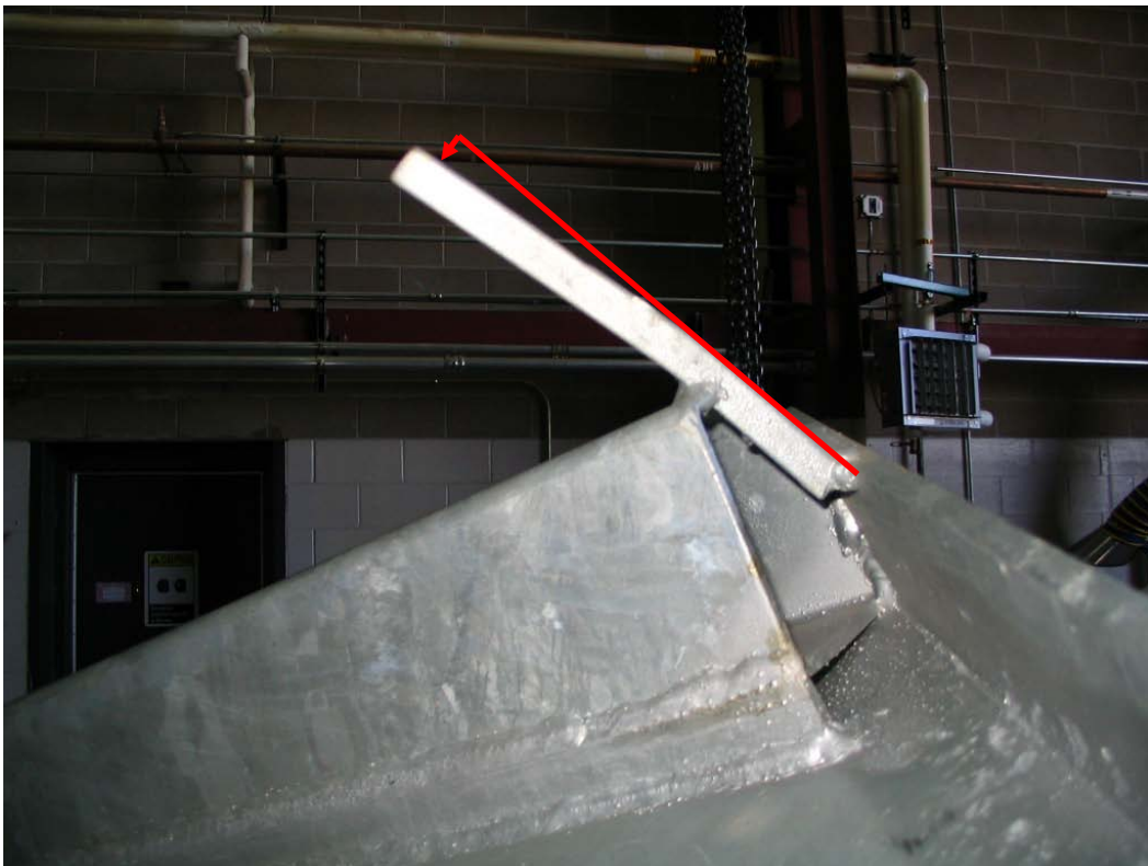
Figure C-14. Bent furl stop
