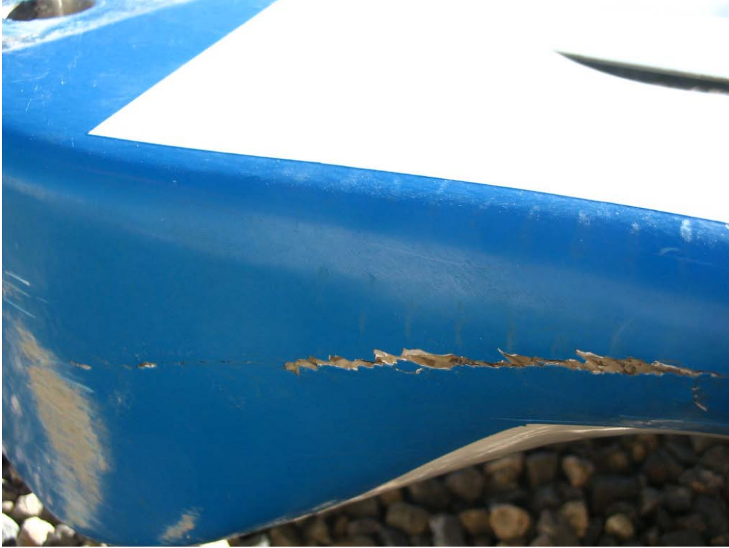
Figure C-11. Crack in leading edge near blade root of blade #2.
