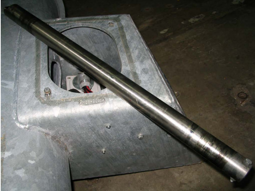
Figure C-15. Tail hinge pin
