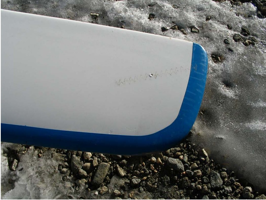
Figure C-9. Remnants of trip strip on one of the blade tips
