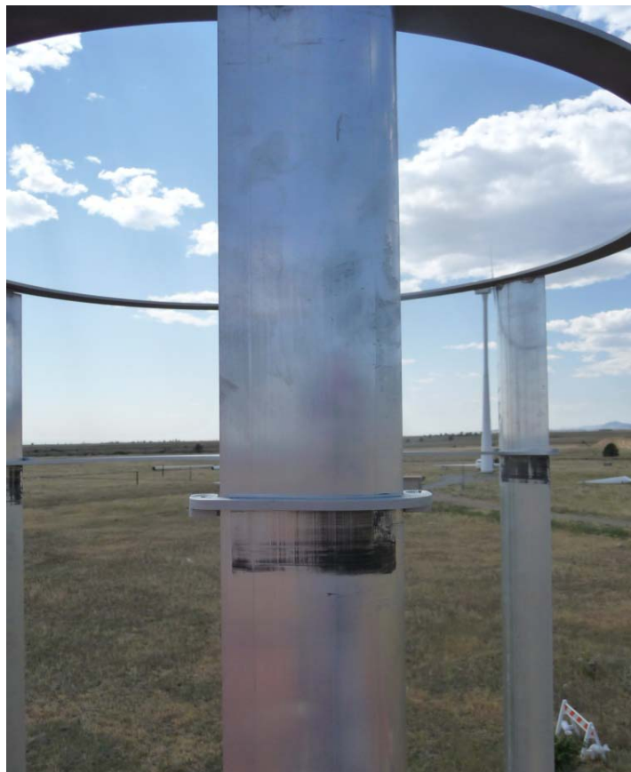
Figure 9. Evidence of airfoil movement in struts
