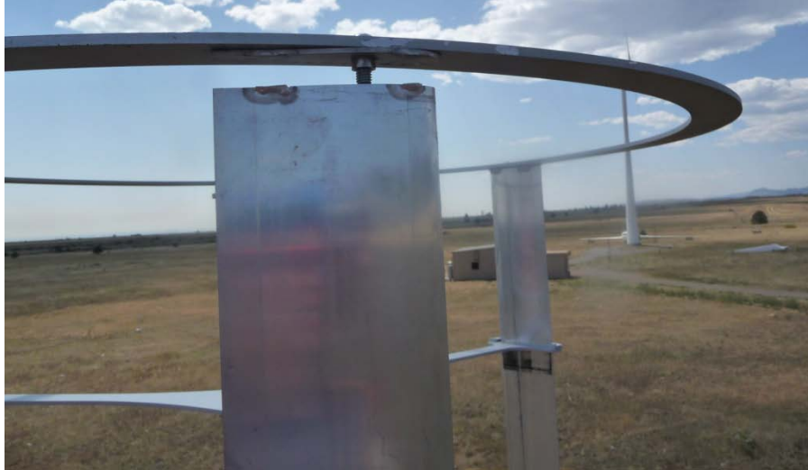
Figure 8. Separated weld between airfoil and cap
