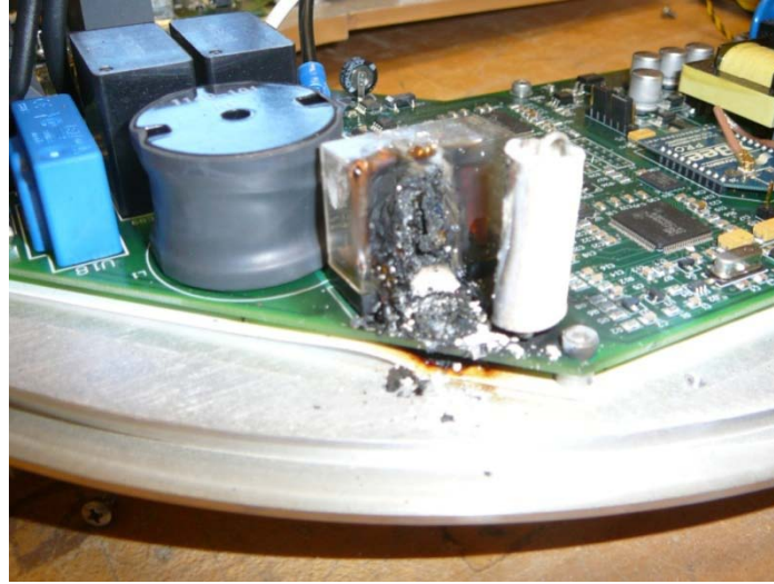
Figure 5. Damaged electrical components in the inverter
