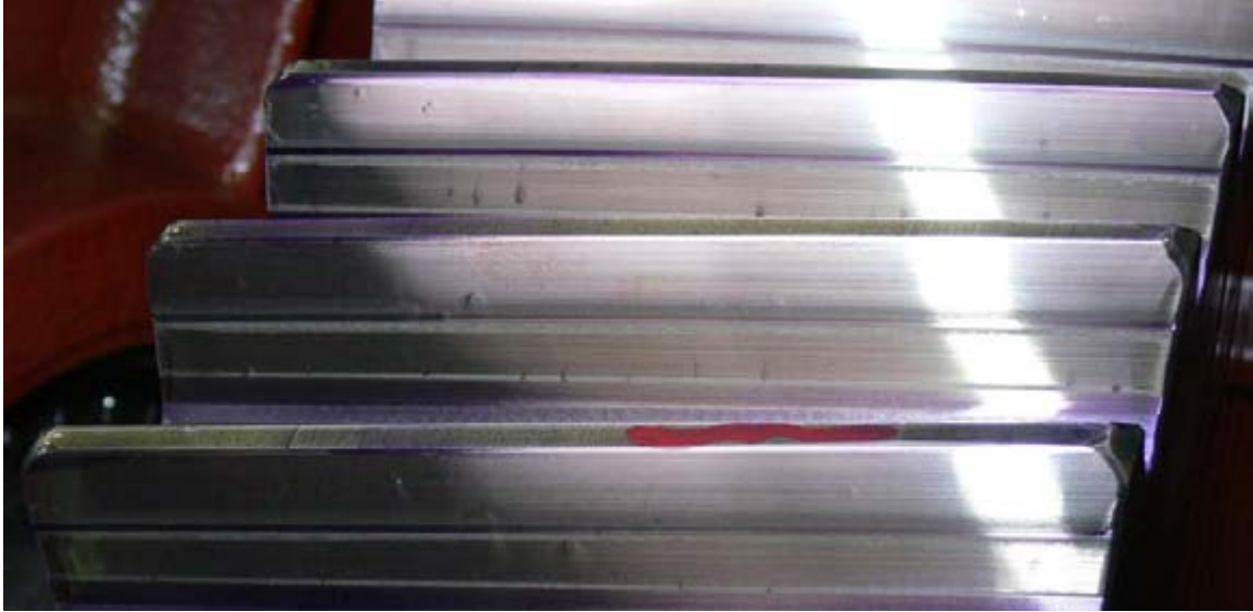
Figure O.23. Convoloid low speed gear after 763 total test hours; light micropitting is visible at the edges of the dedendum side of the transition zone; no micropitting is evident at the tip, nor is there much bluing
