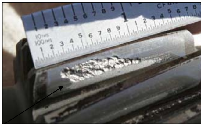
Figure 7.8. Massive macropitting on pinion tooth flank (Test 3, gearbox 2, pinion 1)
