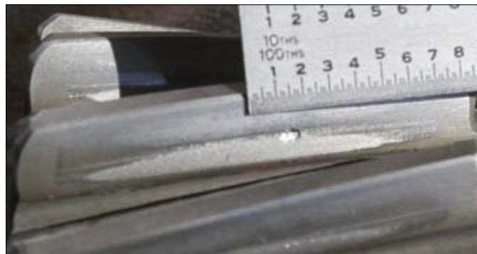
Figure A.29. Failed involute pinion from Test 4
