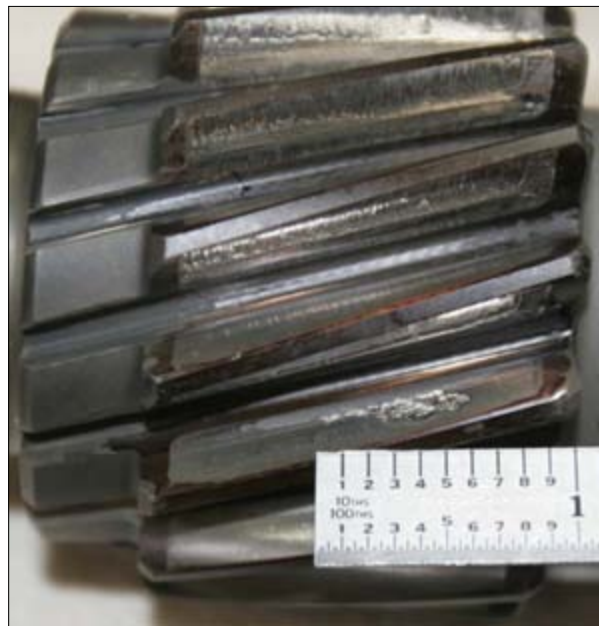
Figure 7.10. Further pitting and opposite flank scuffing damage from Test 2
