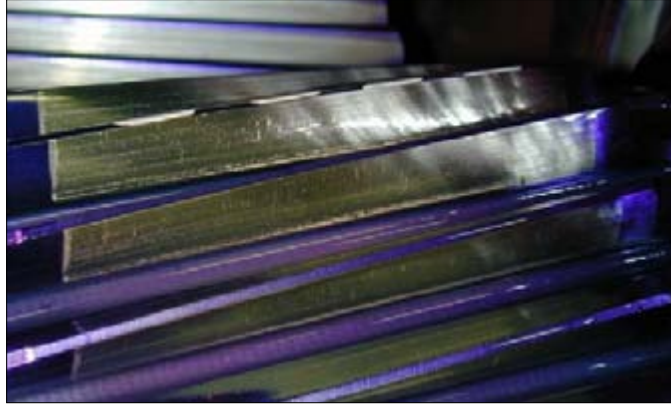
Figure P.10. Involute HS pinion with micropitting in the dedendum and edge distress (true 200% load after 21.9 hours)
