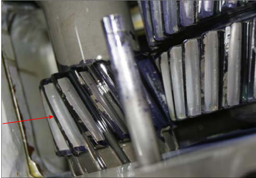
Figure A.23. Involute pinion 2—increaser operation (gear drives pinion)—shows a smaller amount of micropitting on the pinion (arrow) as well as on the mating gear
