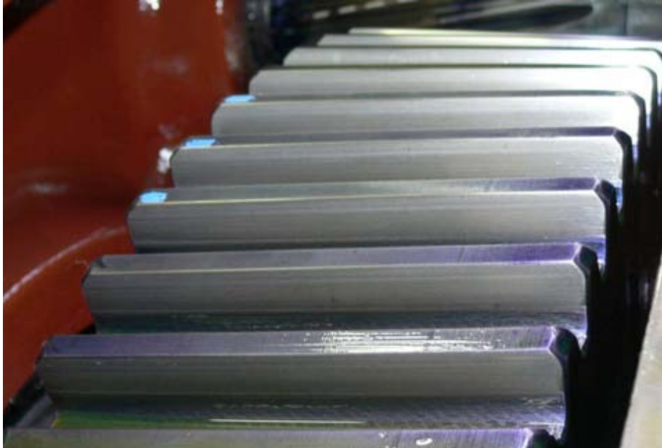
Figure P.43. Involute LS gear at the end of test; no wear is visible (235 hours at 200% load; 528 hours at 240% load)
