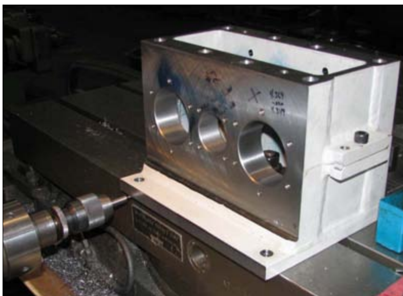
Figure 6.9. The 3-Hole Test gearbox during final machining
