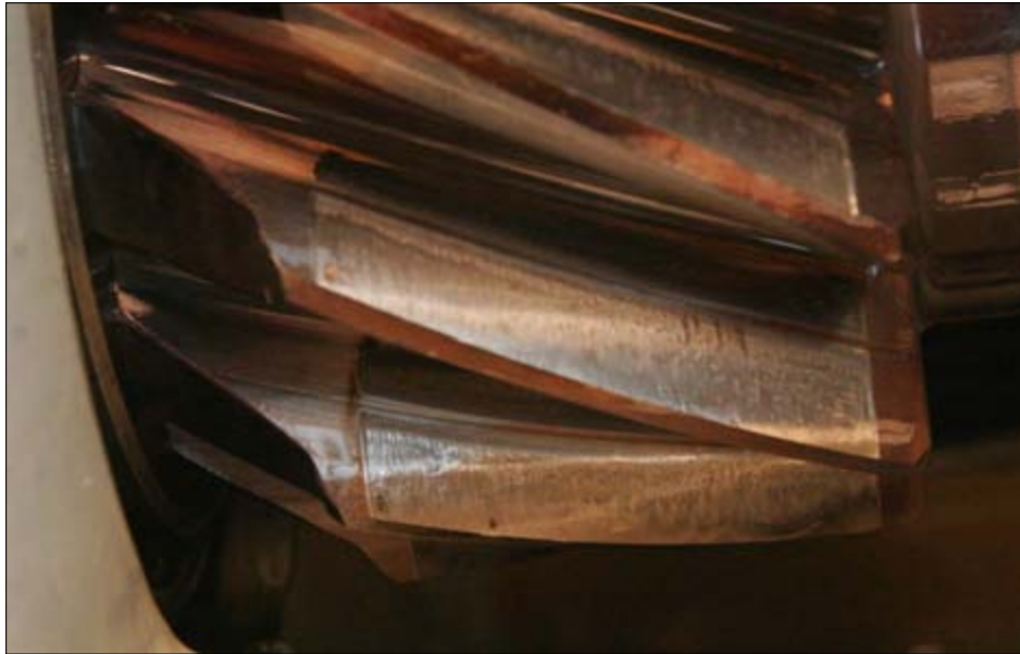
Figure 7.1. Severe scuffing failure due to loss of lubricant
