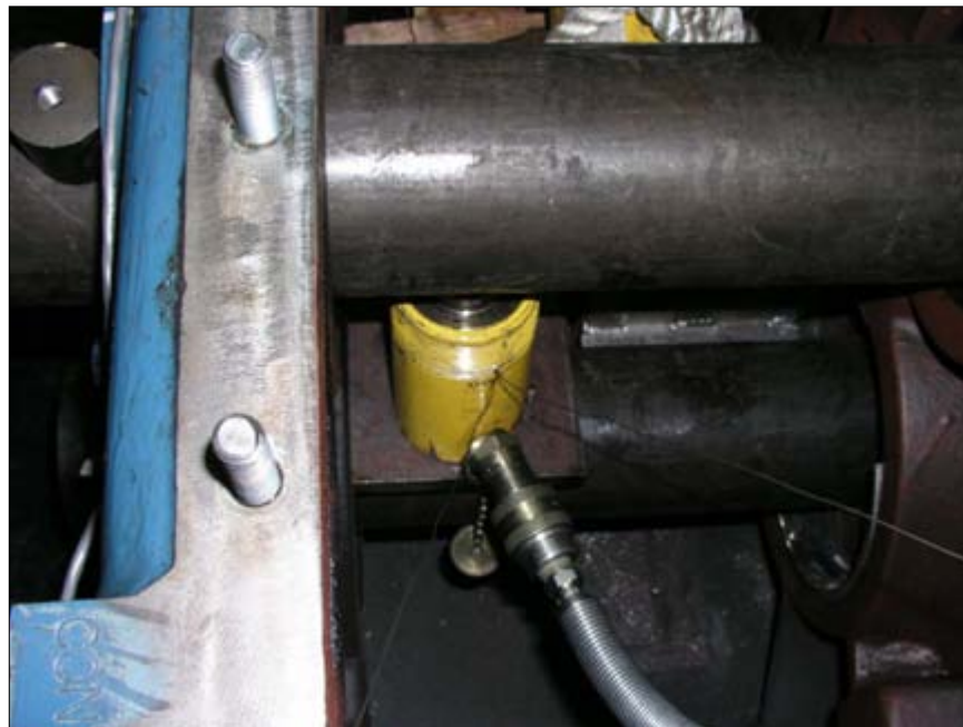
Figure U.2. Close-up of a hydraulic cylinder in position to apply a separating load
