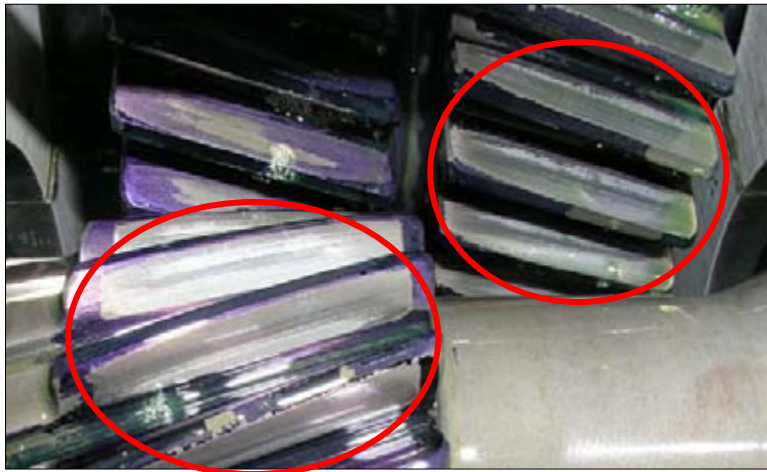
Figure 7.7. Involute gearing showing early micropitting; both parts (circled) drive their respective mates
