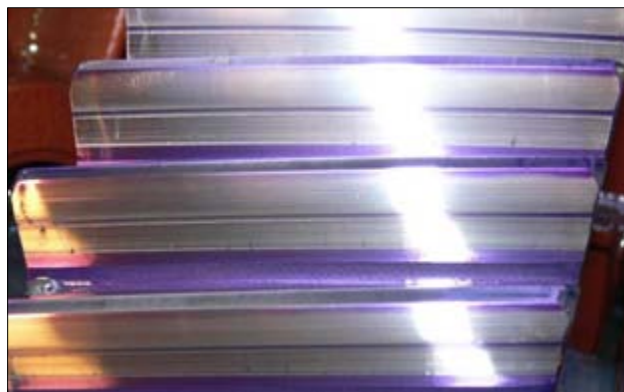
Figure P.27. Convold LS gear at the conclusion of the 200% test; light micropitting is evident around the transition zone and at the root; good tip relief causes the wear pattern to fade away at the tip; 235 hours at 200% load
