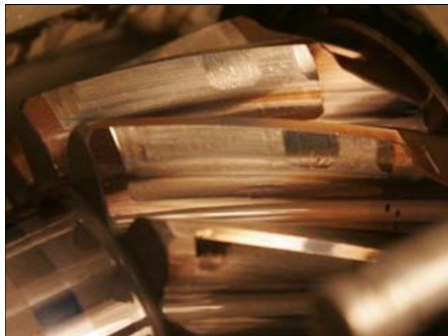
Figure A.12. Severe scuffing on the Convoloid pinions due to loss of lubricant
