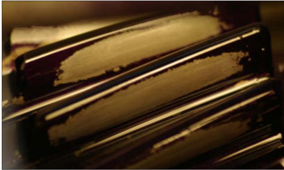
Figure A.18. Representative involute no-load contact
