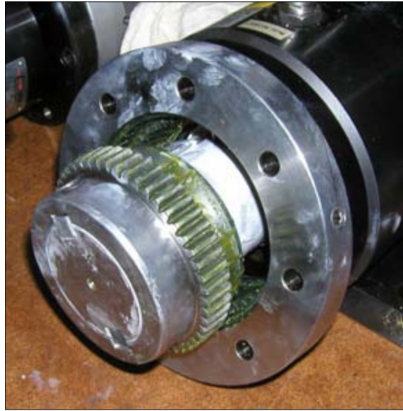
Figure A.9. Flexible half of new coupling
