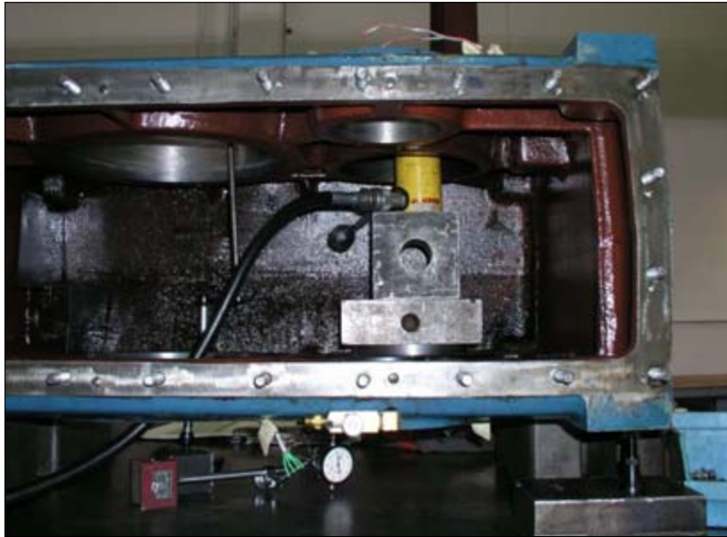
Figure 4.24. Housing stiffness test configuration
