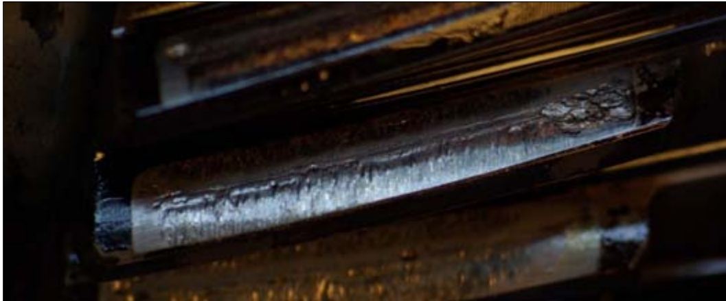
Figure A.24. Involute (1) reducer pinion surface wear (Test 2)
