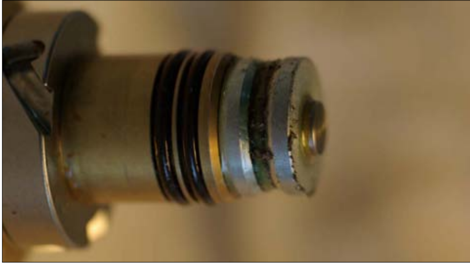
Figure 6.6. One of the chip detectors after a surface fatigue failure
