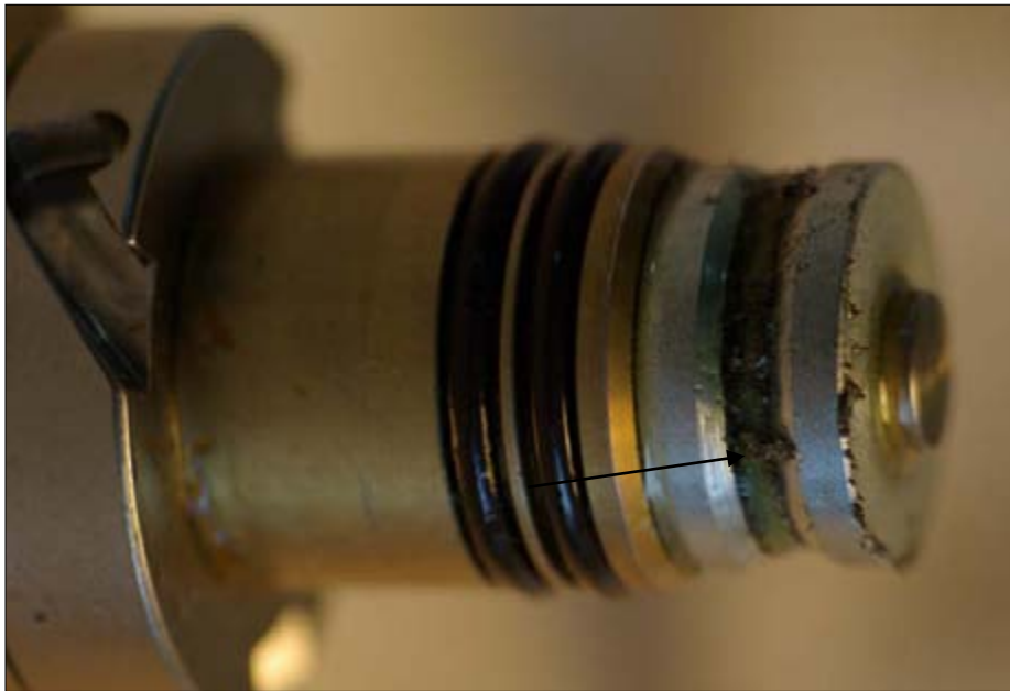
Figure A.25. Gearbox 1 chip detector after gearing failure; note material crossing the gap
