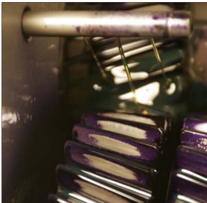
Figure A.20. No-load contact pattern—involute gear; lube nozzle
