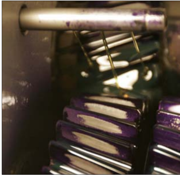
Figure 7.5. No-load contact pattern—involute gear; lube nozzle
