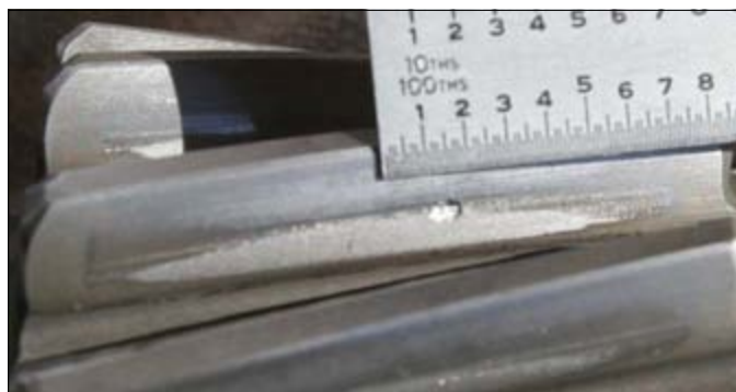
Figure 7.12. Pinion loaded as a speed reducer
