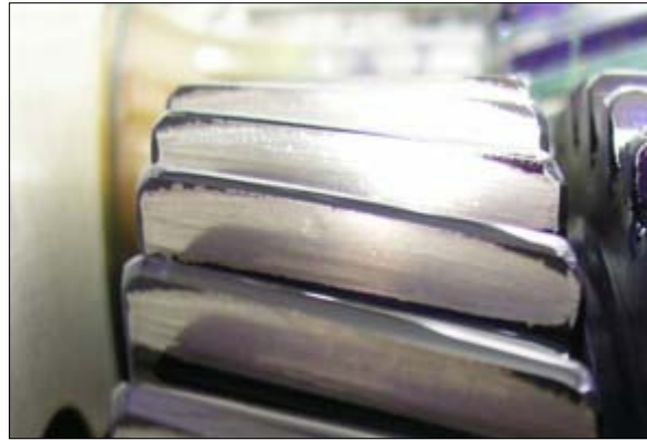
Figure A.21. Example of the full load (7,000 lb-in) contact—involute gears
