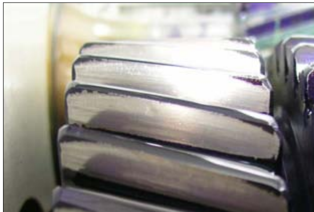
Figure 7.6. Example of the full load (7,000 lb-in) contact—involute gears
