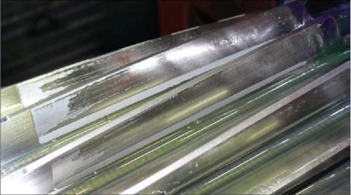
Figure P.37. Involute HS pinion at the end of test; wear due to micropitting is extensive along one side (235 hours at 200% load; 528 hours at 240% load)
