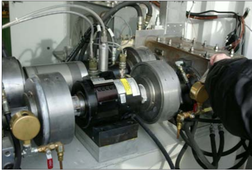
Figure A.7. The 3-Hole Test fixture showing couplings with alignment covers
