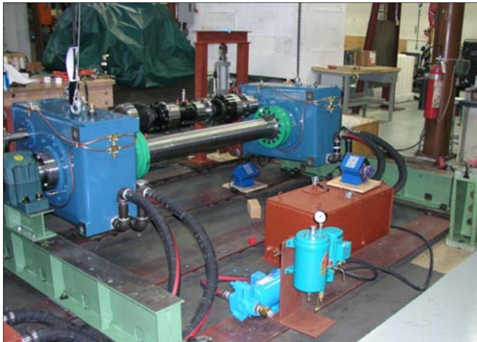
Figure 2.2. Micon 108 test fixture, involute gearbox on the left and Convoloid gearbox on the right
