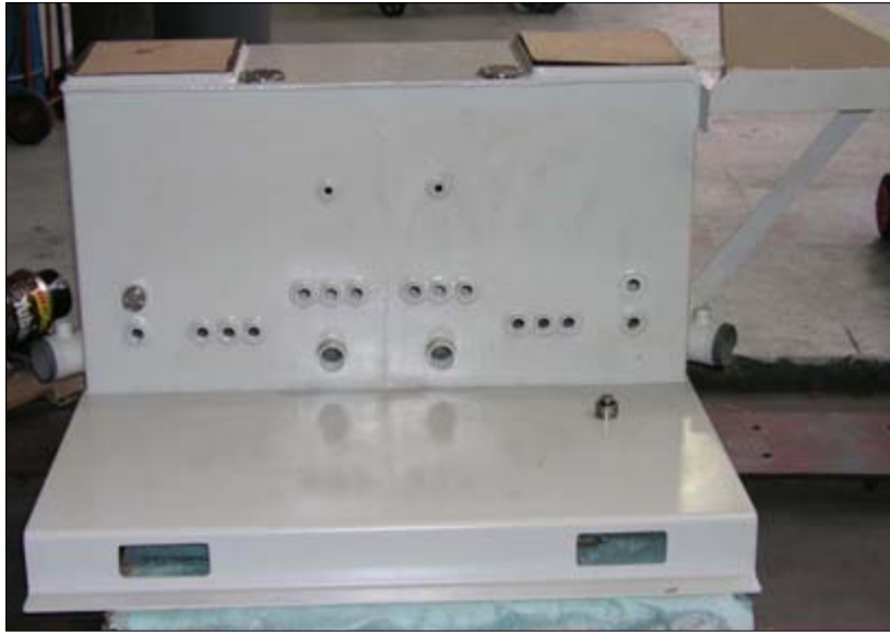
Figure A.2. The 3-Hole Test fixture after paint and initial top milling
