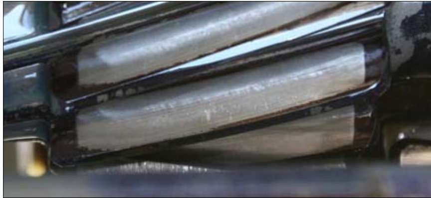
Figure A.31. The other pinion in the same gearbox loaded as a speed increaser showing minimal wear
