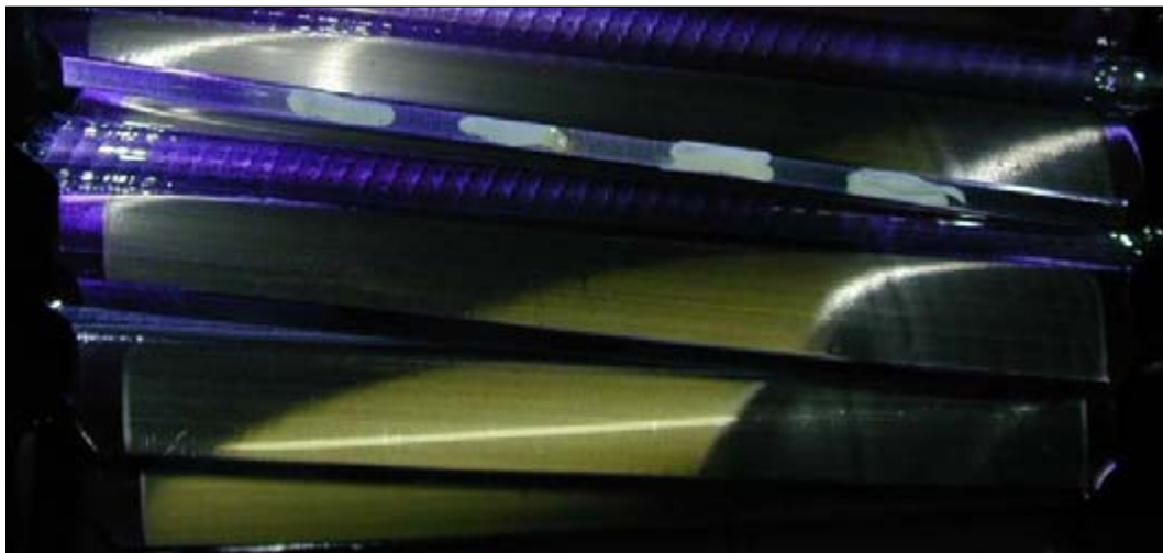
Figure O.7. Involute low speed pinion at 200% shakedown; the contact patch reveals a consistent contact pattern across the contact flank; note paint marks on teeth tips for inspection purposes
