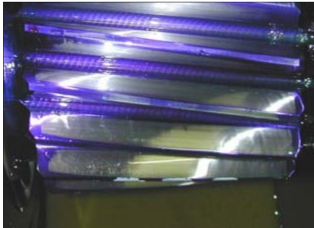
Figure P.5. LS Involute, 77% shakedown contact
