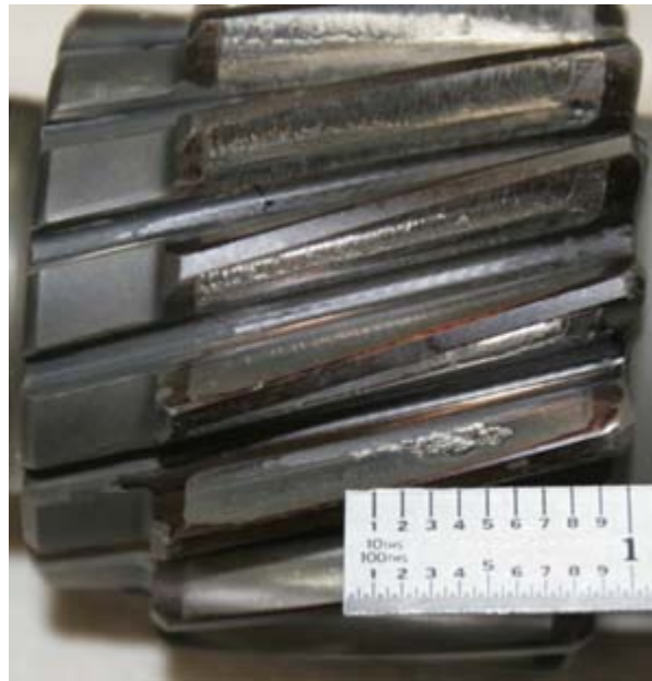
Figure A.28. Further pitting and opposite flank scuffing damage from Test 2
