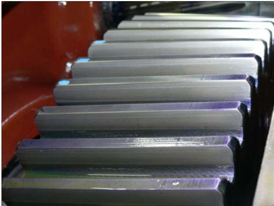
Figure 4.21. Involute LS gear at the end of test; no wear is visible (235 hours at 200% load; 528 hours at 240% load)
