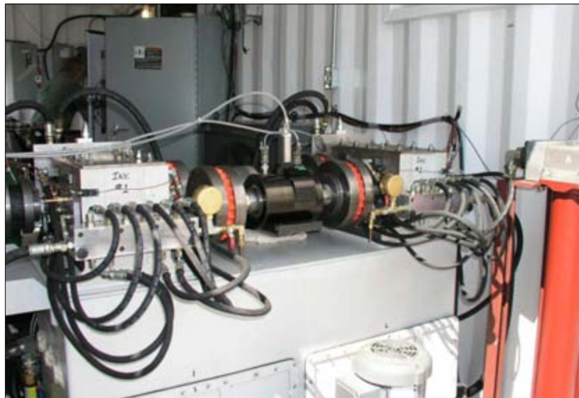
Figure A.6. Initial assembly of 3-Hole Test fixture
