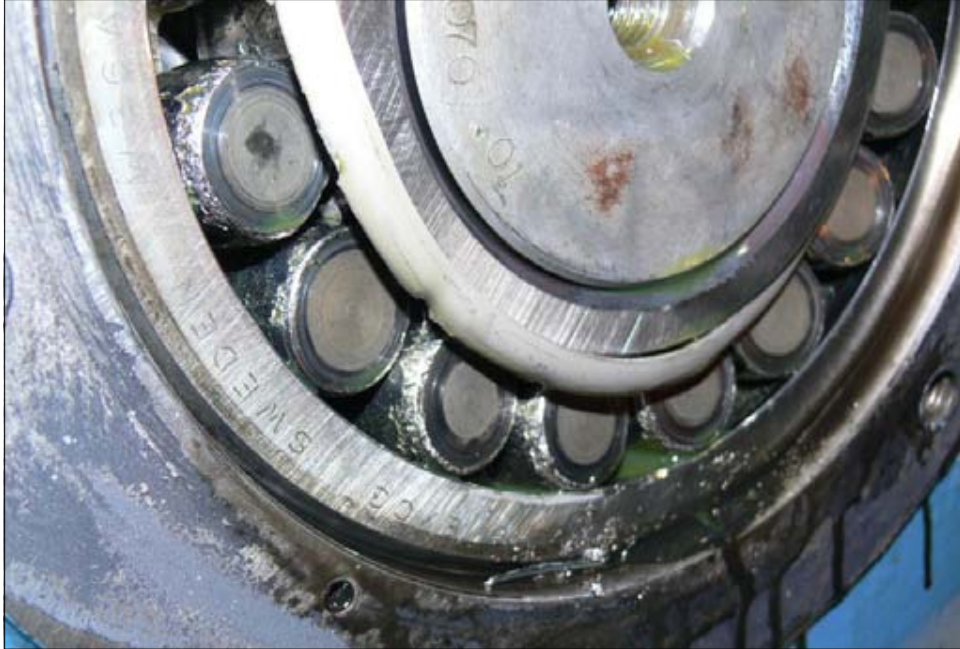
Figure O.24. Failed spherical roller bearing in Convoloid gearbox after 763 total test hours; note pitted edges of the rollers and deformation of the cage; metallic particles are present at the bottom of the housing bore
