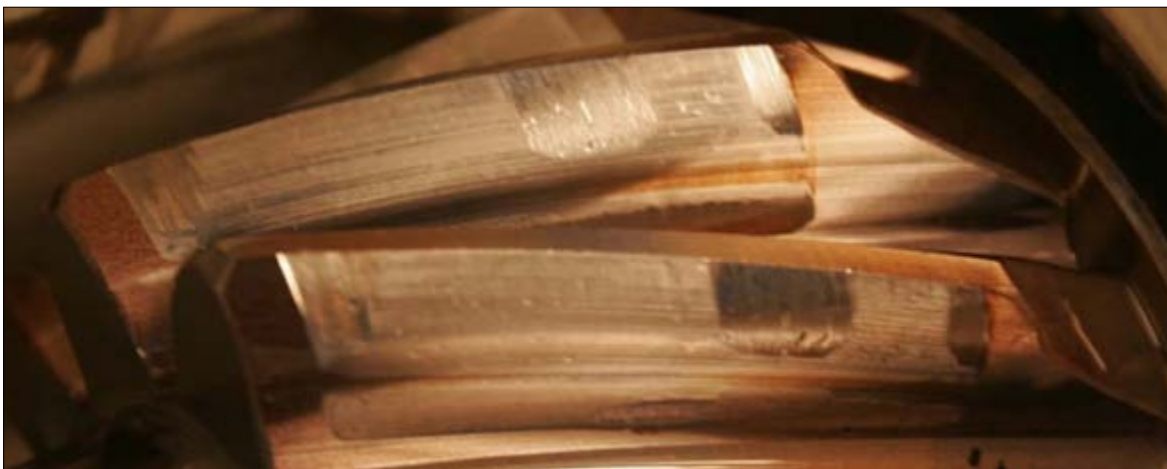
Figure 7.3. Close-up of Convoloid gear tooth with no micropitting and partial scuffing damage due to loss of lubrication
