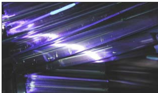
Figure P.6. HS Convoloid, 77% shakedown contact
