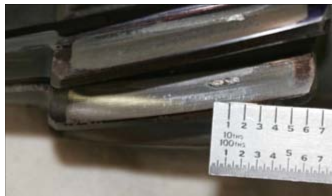
Figure A.27. Additional pitting flank (Test 3, gearbox 2, pinion 1)
