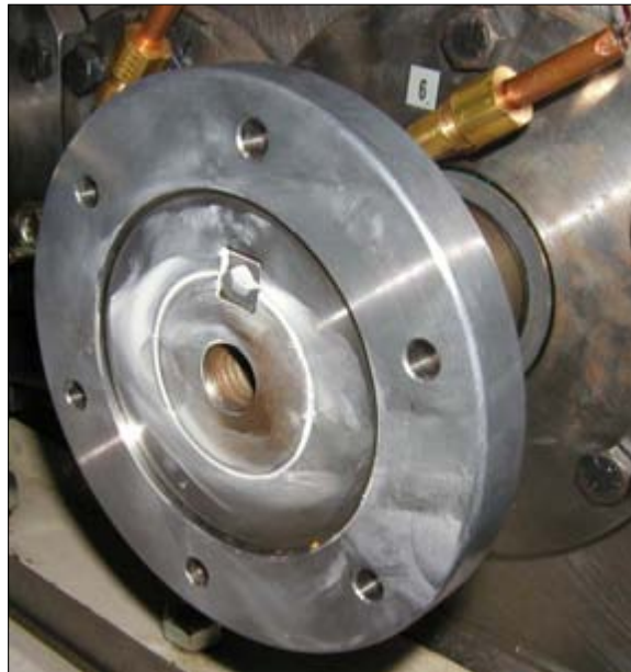
Figure A.8. Fixed half of new coupling
