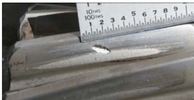
Figure 7.11. Failed involute pinion from Test 4
