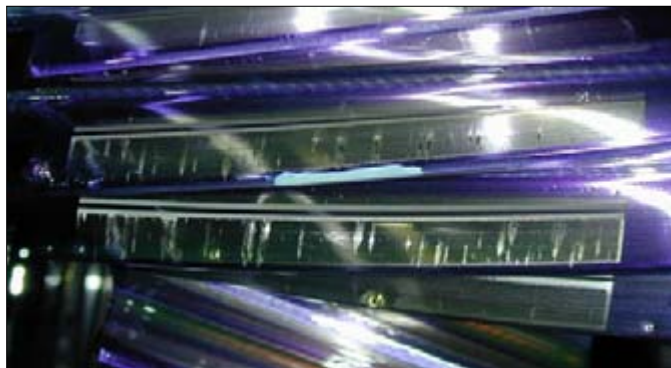
Figure P.12. Convoloid HS pinion with full face contact, showing transition zone micropitting and edge distress (21.9 hours at 200% load)
