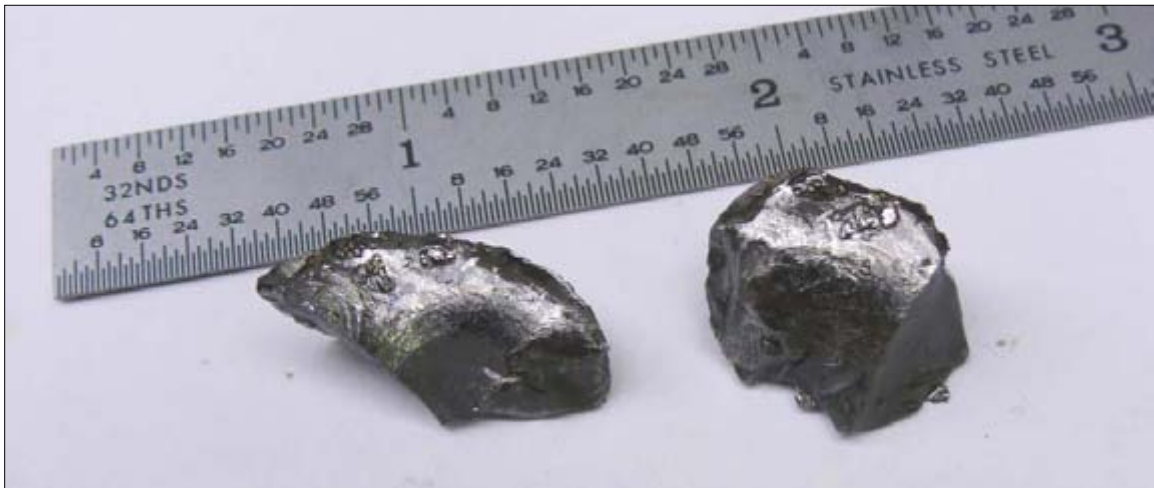
Figure O.25. Pieces of the failed bearing
