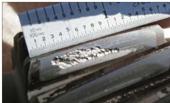
Figure A.26. Massive macropitting on pinion tooth
