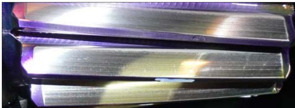
Figure O.8. Involute low speed pinion after 235 hours at 200% rated load; light micropitting is visible on all four edges of contact with a heavier concentration in the dedendum; faint micropitting also is visible on the grinding peaks (faint lines that run horizontal in the active flank)
