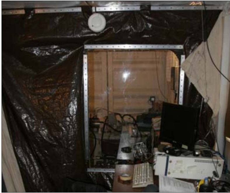
Figure A.5. View inside the test container showing the computer monitoring system and polycarbonate view window
