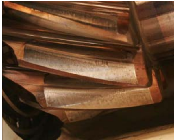
Figure A.11. Severe scuffing on the Convoloid pinions due to loss of lubricant
