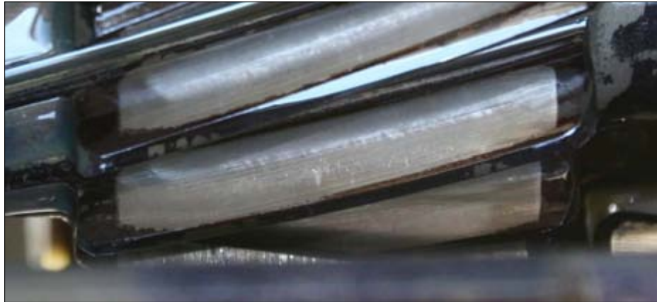
Figure 7.13. The other pinion in the same gearbox loaded as a speed increaser and showing minimal wear
