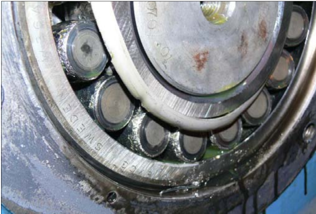
Figure 4.11. Failed spherical roller bearing in Convoloid gearbox after 763 total test hours; note pitted edges of the rollers and deformation of the cage; metallic particles are present at the bottom of the housing bore
