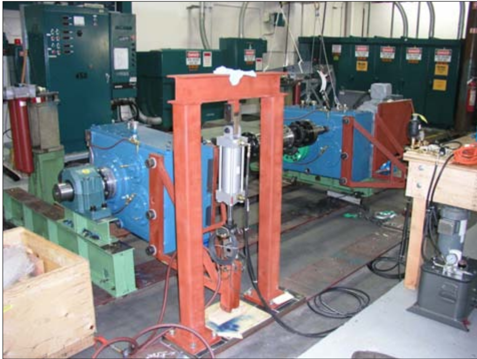
Figure 2.3. Micon 108 test fixture, Convolid gearbox with torque application hydraulic cylinder
