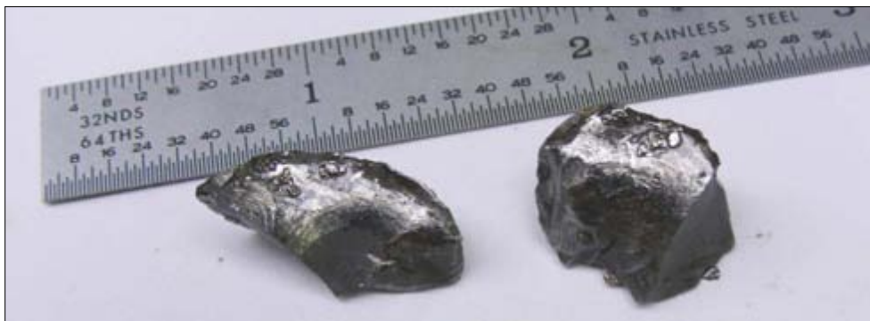
Figure 4.12. Pieces of the failed bearing
