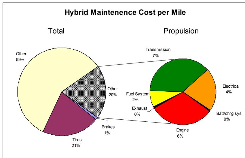
**Figure 14. Propulsion maintenance cost per mile (hybrids)**
