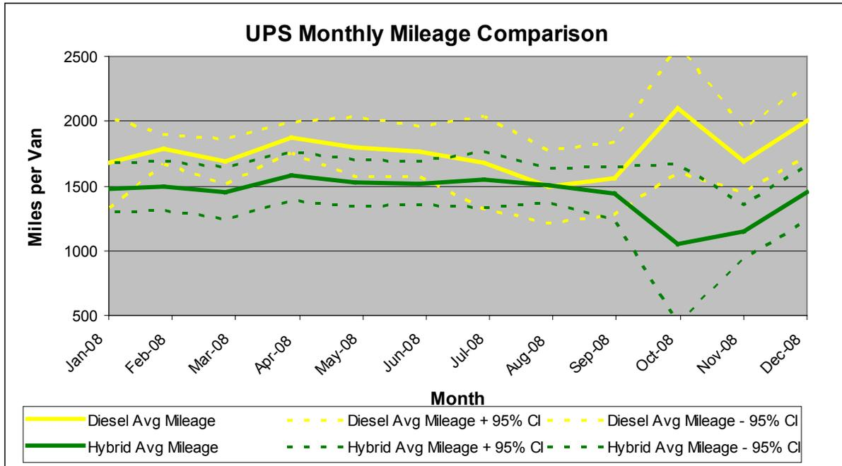
**Figure 6. Hybrid and diesel monthly mileage per van**
