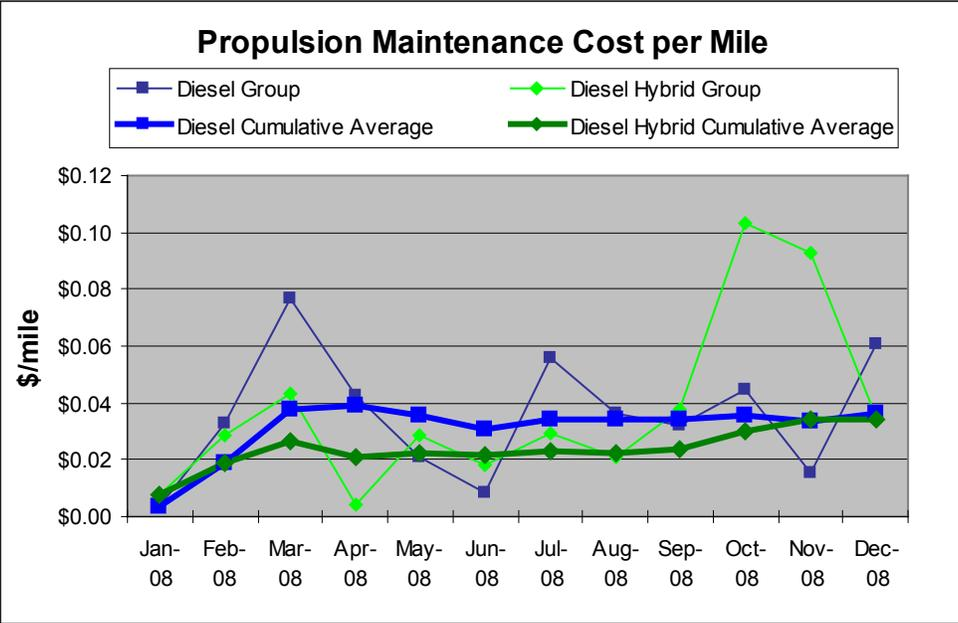
**Figure 12. Propulsion maintenance cost per mile**
