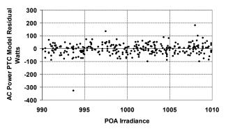
Fig. 3. Residuals (measured – modeled) of measured data from the PVUSA TC model line for irradiance levels from 990 Wm<sup>-2</sup> to 1000 Wm<sup>-2</sup>. Note this includes temperature range from -32.5 °C to 36 °C and wind speeds from 0.4 to 9.1 ms<sup>-1</sup>.
