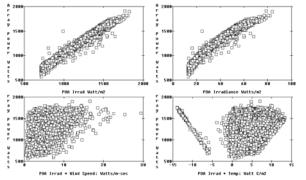
Fig. 5. Correlations of array power with each independent term of the PVUSA TC model. Top left to bottom right: array power versus a\*I,  $b*I^2$ , c\*I\*w, d\*I\*T. The values of a, b, c, and d developed from the model are used. Note the lack of strong correlation between wind speed and temperature components of the model and the array output, except for very cold (T<-5 °C) day [135 data points] in the bottom right graph.
