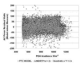
Fig. 6. Residuals between measured and modeled PTC (gray squares), and quadratic (open circle) and linear (+) fits of AC power versus irradiance alone for the USSC system.
