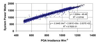
Fig 2. USSC Array data after filtering for non-standard operating conditions and for POA>  $500 \text{ Wm}^{-2}$
