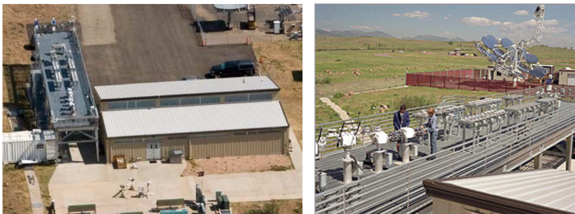
Figure 1-1. General SRRL configuration (left) with instrument platform (oriented north-south) located west of building. North is to the top, east to the right of the photograph. Instrument platform (right) with solar tracking instruments to the left (south) and horizontal instruments to right (north).
