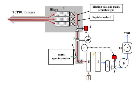
Figure 4: Schematic of TMBMS gas sampling system: (1) sampling manifold; (2) flow-control valve; (3) orifice-plate flow meter; (4) sampling orifice; (5) condenser; (6) chilled impingers with cotton wool; (7) coalescing filter; (8) pressure control valve; (9) sample pump; (10) dry test meter. Shaded areas maintained at 450°C.
