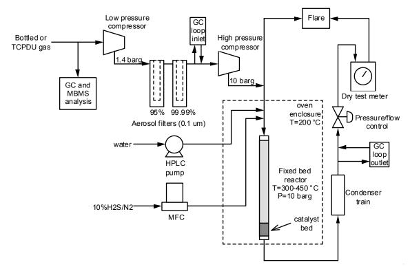
Figure 3: Schematic of fixed bed reactor system (BTRS, Jr.)
