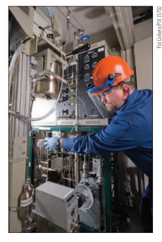
Catalytic fuels synthesis unit converts syngas to liquid fuels such as methanol and mixed alcohols.
