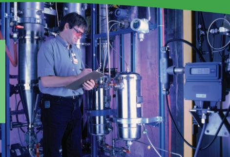
The scrubbers on the TCPDU are used to remove the steam and condensable tars from the synthesis gas.
