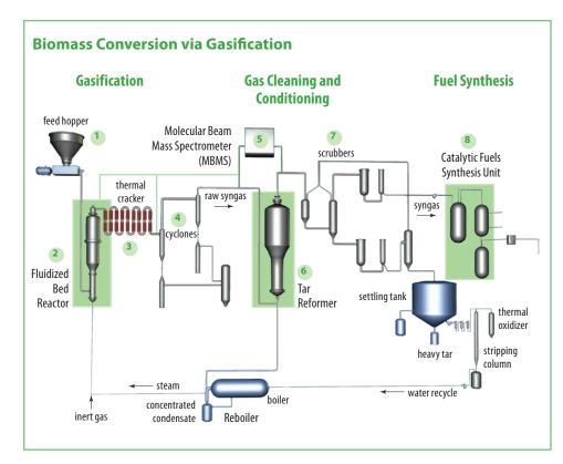
This figure illustrates biomass gasification in a fluidized bed reactor.
