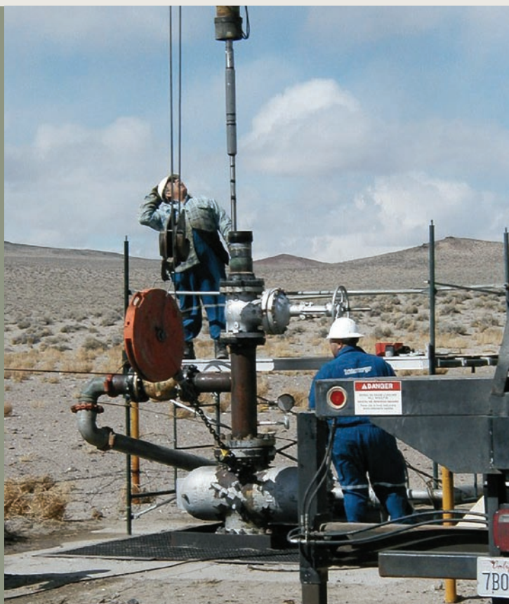
Drilling exploration crew performing initial well logging tests at the Desert Peak site in Nevada.
