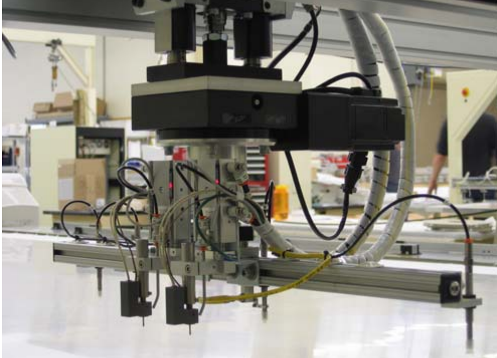
Figure 49 Robot end effector with soldering heads and vacuum pick-up arm.
