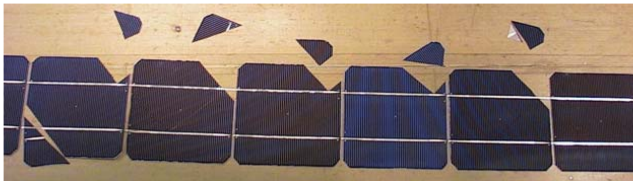
Figure 70 String of 220\ \mu\text{m} cells soldered with 178\ \mu\text{m} thick flat copper ribbons and flexed to show crack locations.
