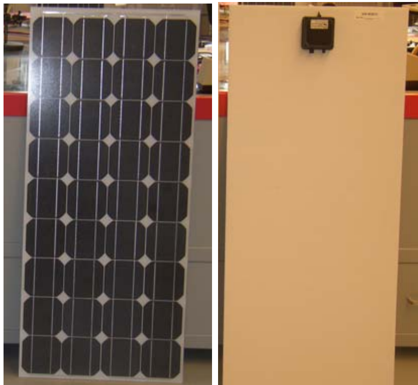
Figure 26 Module laminate made with faster-curing EVA.
