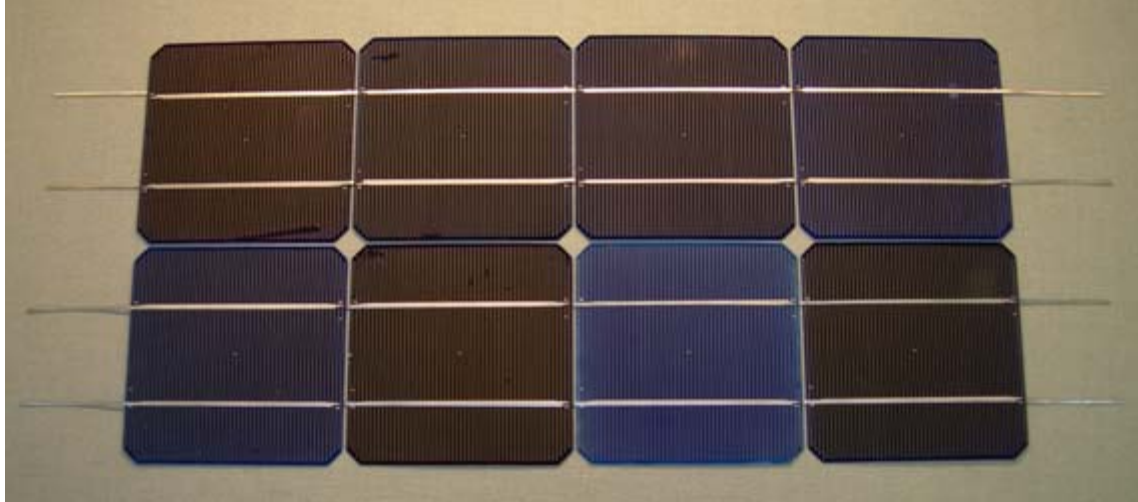
Figure 71 Cell strings made with 220 \mu\text{m} thin cells and 178 \mu\text{m} thick corrugated interconnect ribbons.
