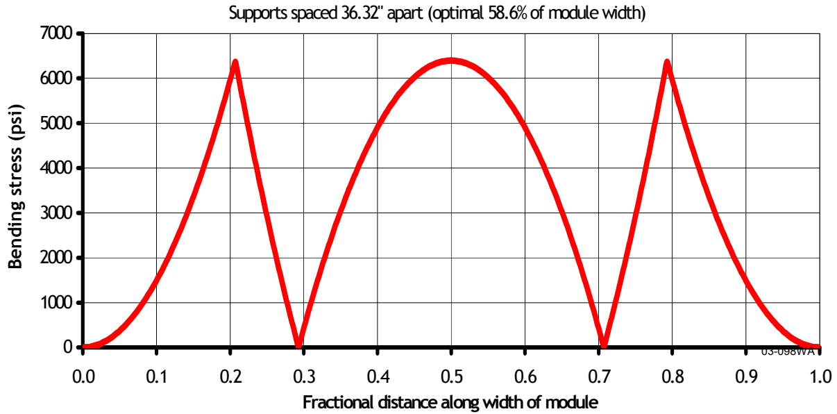
Figure 6 Bending stress profile under maximum wind and snow load (113 psf) for a 1575 mm wide module with a 6.3 mm thick cantilevered single glass sheet.
