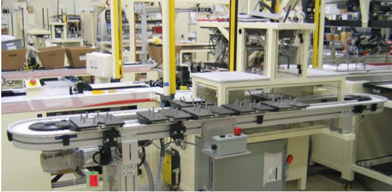
Figure 97 Cell pallet conveyor installed on an automated cell stinging machine.
