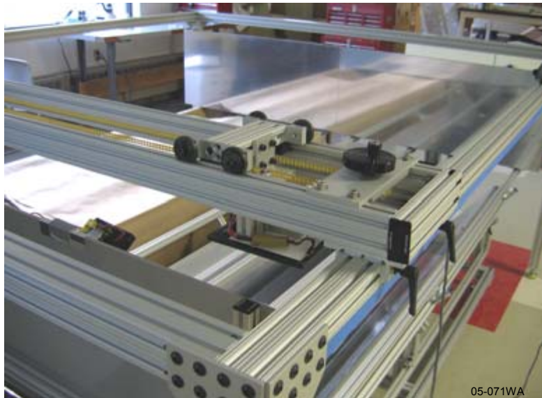
Figure 69 Monitor cell gantry for measuring light uniformity over a 2 m x 2 m test area.
