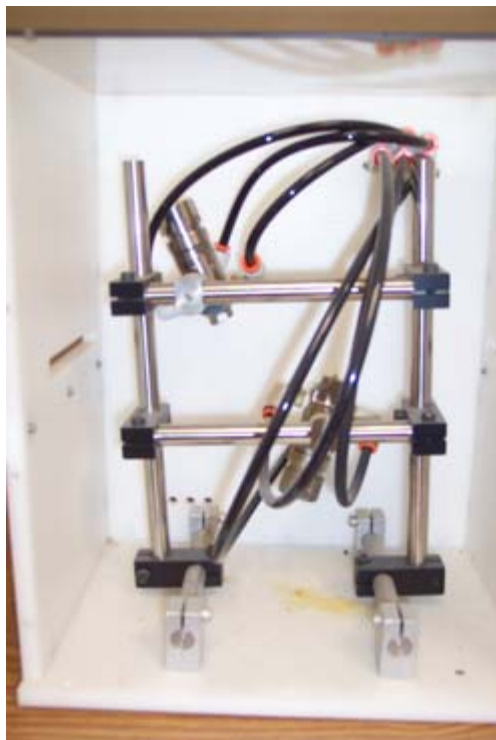
Figure 95 Prototype flux spray applicator assembly.
