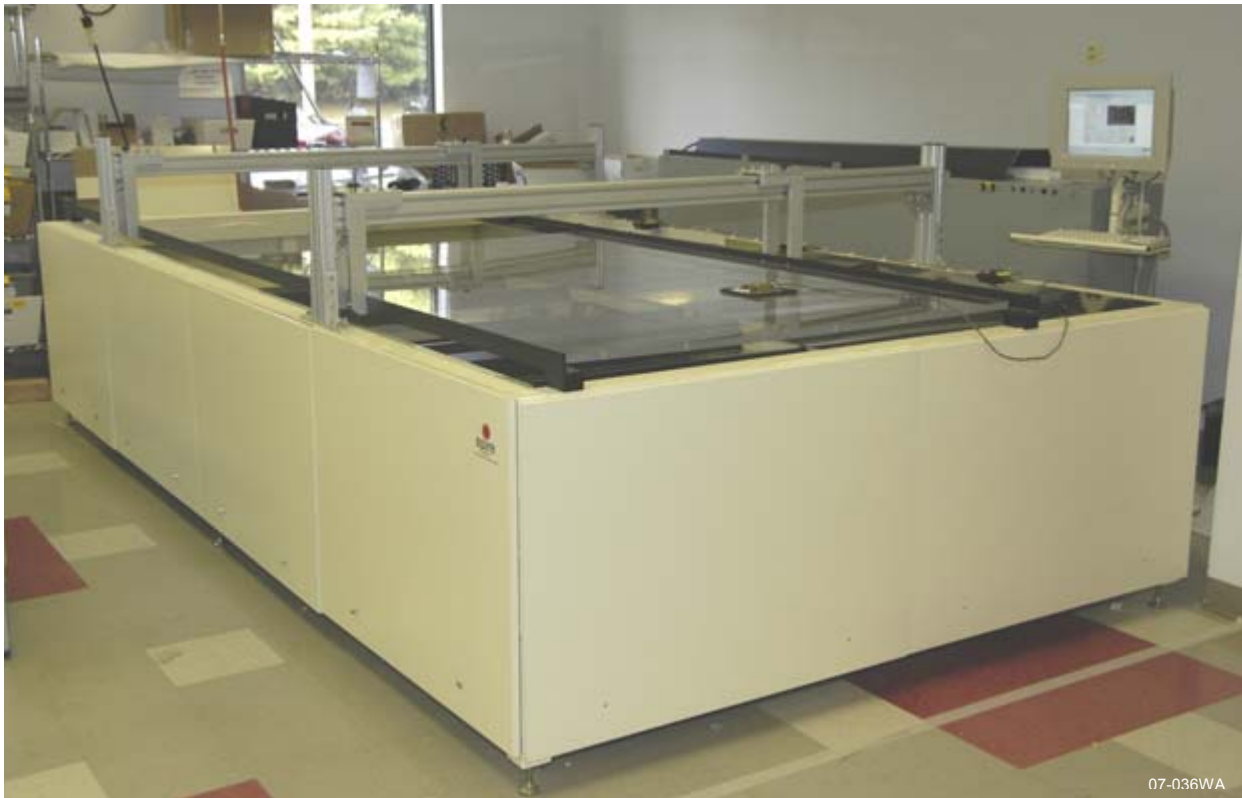
Figure 79 Spi-Sun Simulator 2040SLP, set up for spatial uniformity testing.
