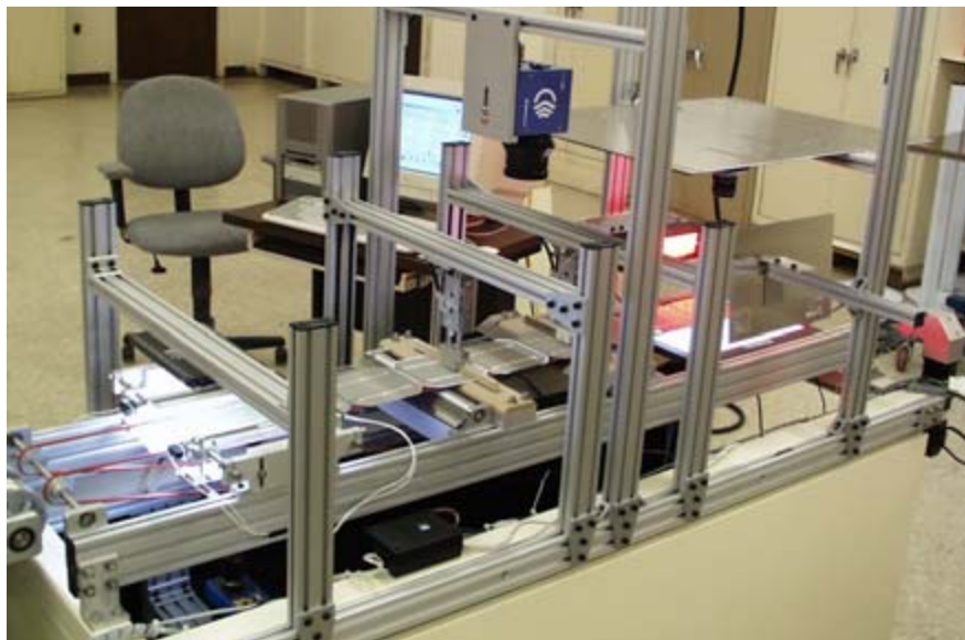
Figure 24 Cell string inspection system with a string of 125 mm cells.
