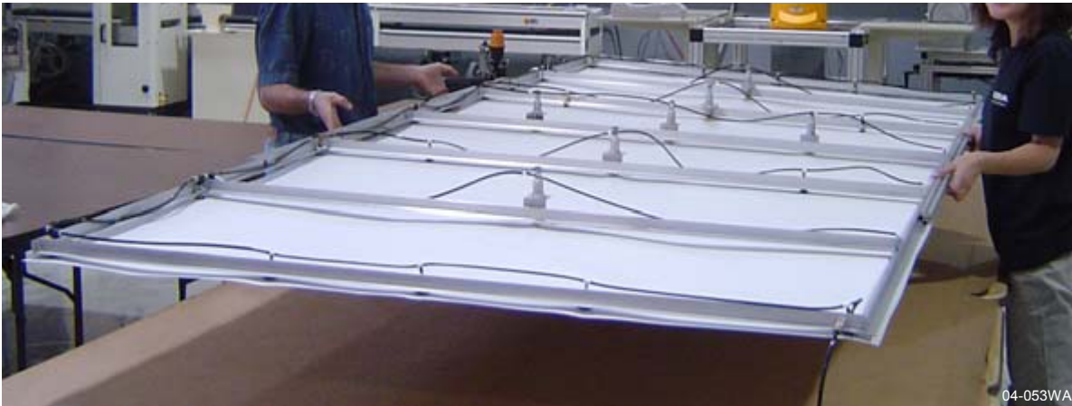
Figure 29 Tedlar sheet (5' x 12') lifted by a vacuum end effector.
