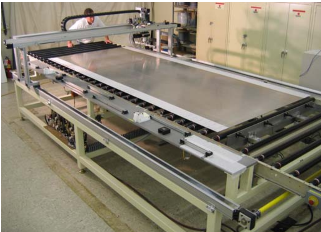
Figure 50 Module-size aluminum sheet on the automated busing system.
