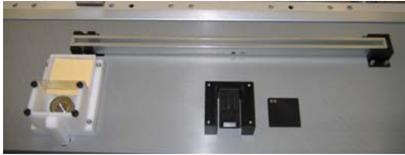
Figure 51 Bus ribbon tray (top), flux applicator (left), and diode pack retainer (center) on front tooling plate.
