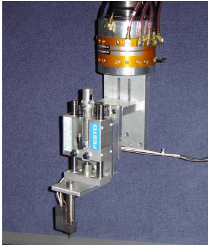
Figure 53 Slide-mounted solder head suspended from robot arm.
