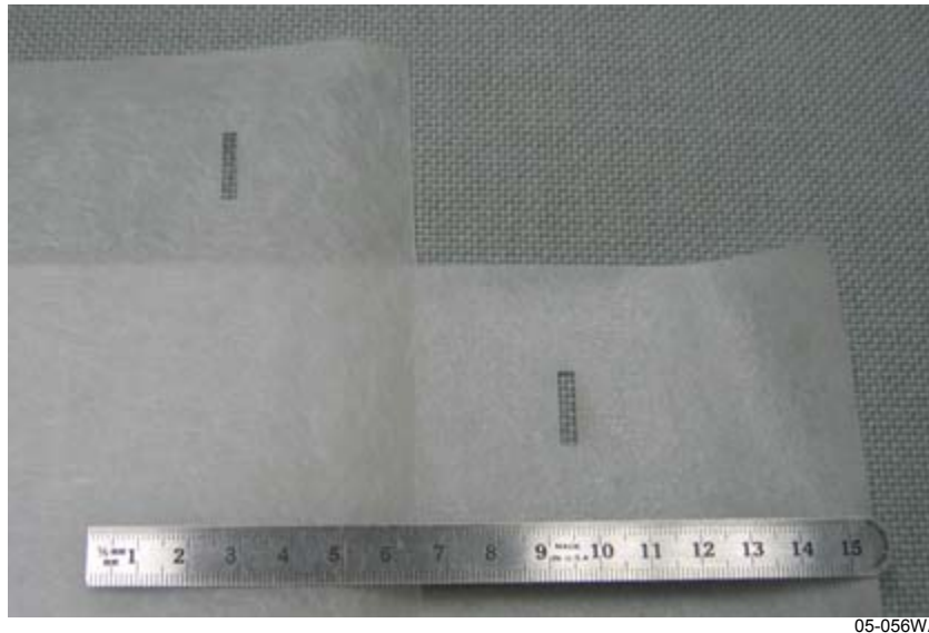
Figure 45 Punched slots in EVA-on-fiberglass sheet.
