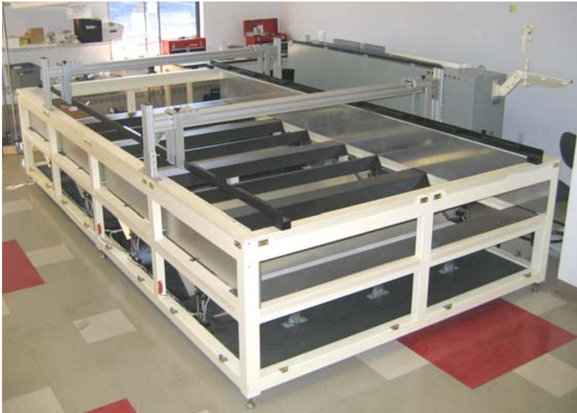
Figure 77 Module support rails mounted on Spi-Sun Simulator 2040SLP.
