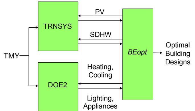
Fig. 2: Optimization with multiple simulation engines
